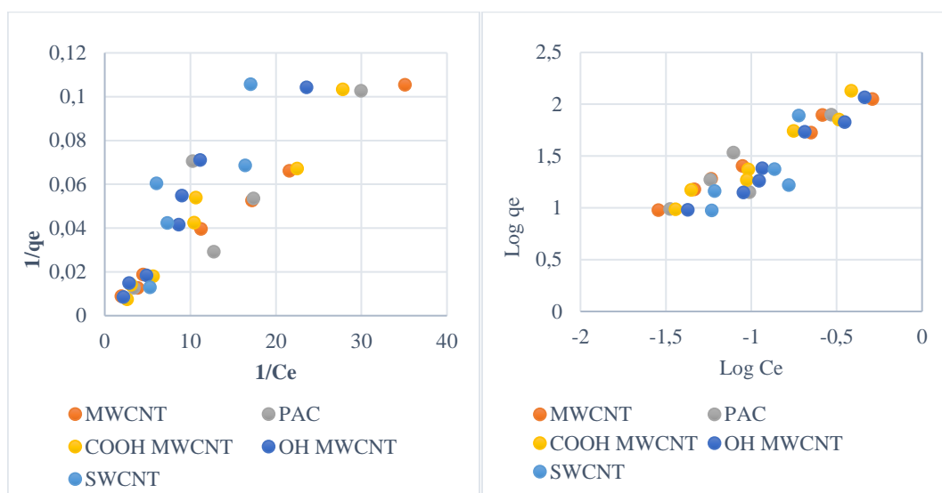
Figure 20. Langmuir and Freundlich Isotherm Plots for the Adsorbents Tested for Aclonifen Adsorption
