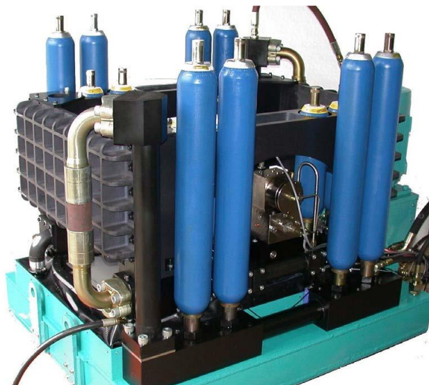
Figure 4.8. Earthquake Simulator (C-CORE)
