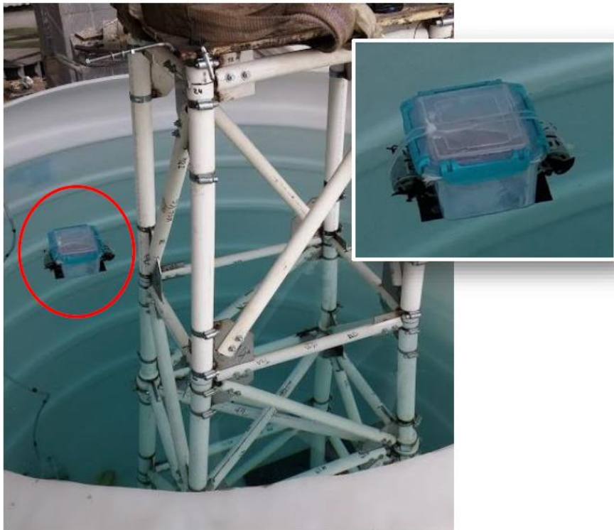
Figure 4.3. When Testing the Underwater Monitoring Device in the Pool
