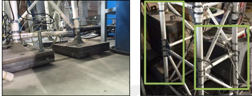
Figure 3.7. Lifting of the Feet and Fixing with Additional Weight
