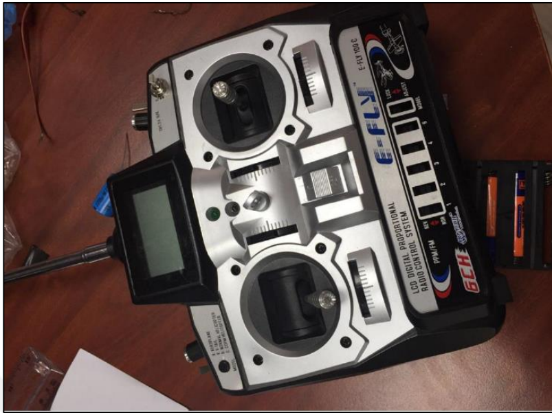
Figure 4.2. Remote Control Device to Control the Underwater Monitoring Device
