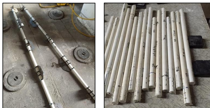
Figure 3.4 Vertical Members and PVC Pipes Used as Horizontal and Diagonal Members
