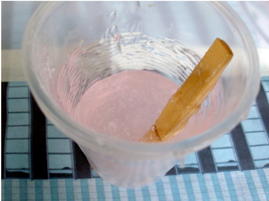
Figure 20. Cold silicon is thinned with toluene.
