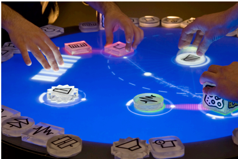
Figure 11. Reactable is collaborative electronic music instrument with a tabletop tangible multi-touch interface. http://mtg.upf.edu (accessed: January 14, 2009)
