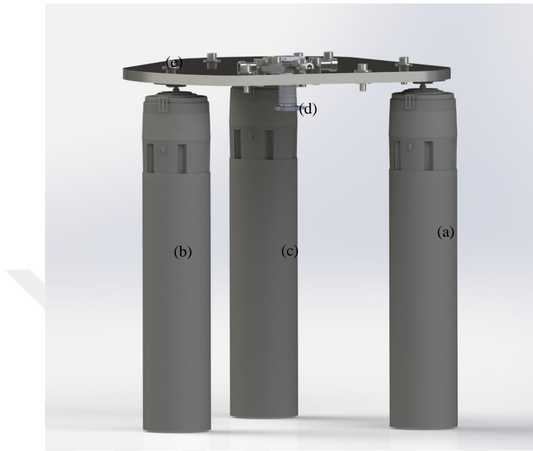
Figure 5. 7 The vibration isolation table schematic design. (a), (b), and (c) are air damping isolation legs, (d) is an edge welded bellows, (e) platform.
