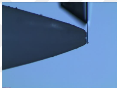
Figure 3. 15 Alignment holder of the cantilever in front of the fiber tubing
