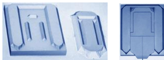
Figure 3. 14 Cantilever Alignment holder chip and cantilever.
