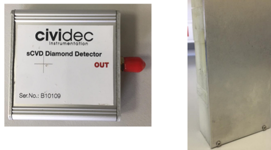
Figure 4.8: Unshielded (left) and shielded (right) diamond detector. The shielding of the detector is Al: 0.25 cm - Pb: 0.40 cm - PE: 0.40 cm from the outside to the inside. Lead and polyethylene layers are embedded inside the light grey aluminum casing. The round detector hole corresponding to the 5.9 mm diameter diamond detector is also visible.
