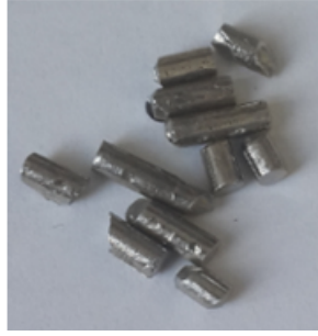
Figure 3.2: Some examples of the produced and cut samples. They were cut by the help of a wire erosion machine due to their brittleness.
