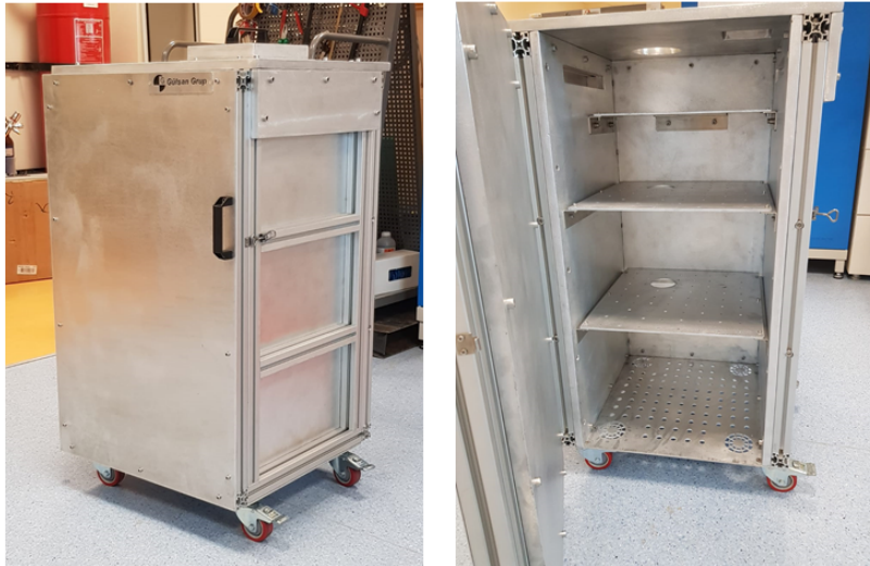
Figure 4.17: The shielding of the second turbomolecular pump from two different angles. The shielding box has a size of 61.0 cm x 59.0 cm x 102.5 cm.
