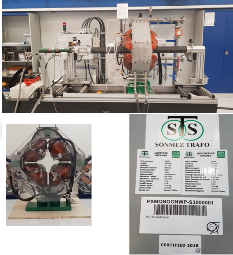
Figure 2.11: The images of third magnet and its certificate from CERN. First image (middle above) is taken at CERN during the magnetic tests of the magnet. The second image (below left) is taken in TAEA PAF and the last image (below right) is the certificate of the magnet from CERN.
