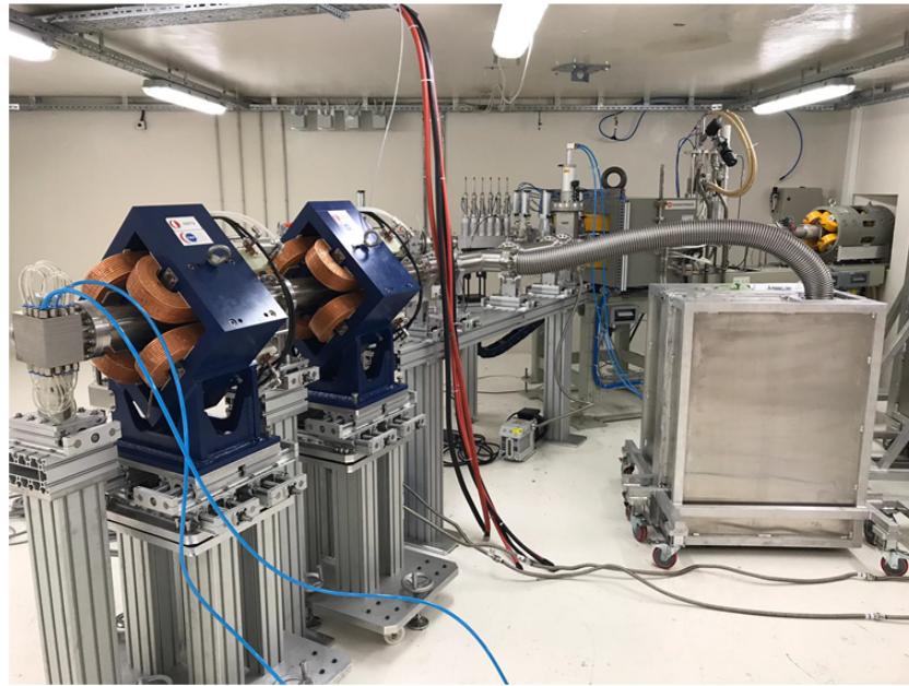
Figure 4.16: The turbomolecular pump (upper panel), connected to the beam pipe with a 1.5 m long and 100 mm wide flex pipe during pretests, and with its shield during the final assembly of METU-DBL (lower panel).
