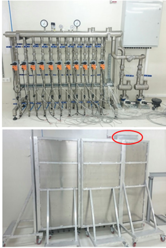
Figure 4.13: Unshielded (above) and shielded (below) cooling subsystem. The shield consists of Al: 0.50 cm - Pb: 0.40 cm - PE: 1.00 cm - Al: 0.25 cm from the outside to the inside and is movable on wheels.
