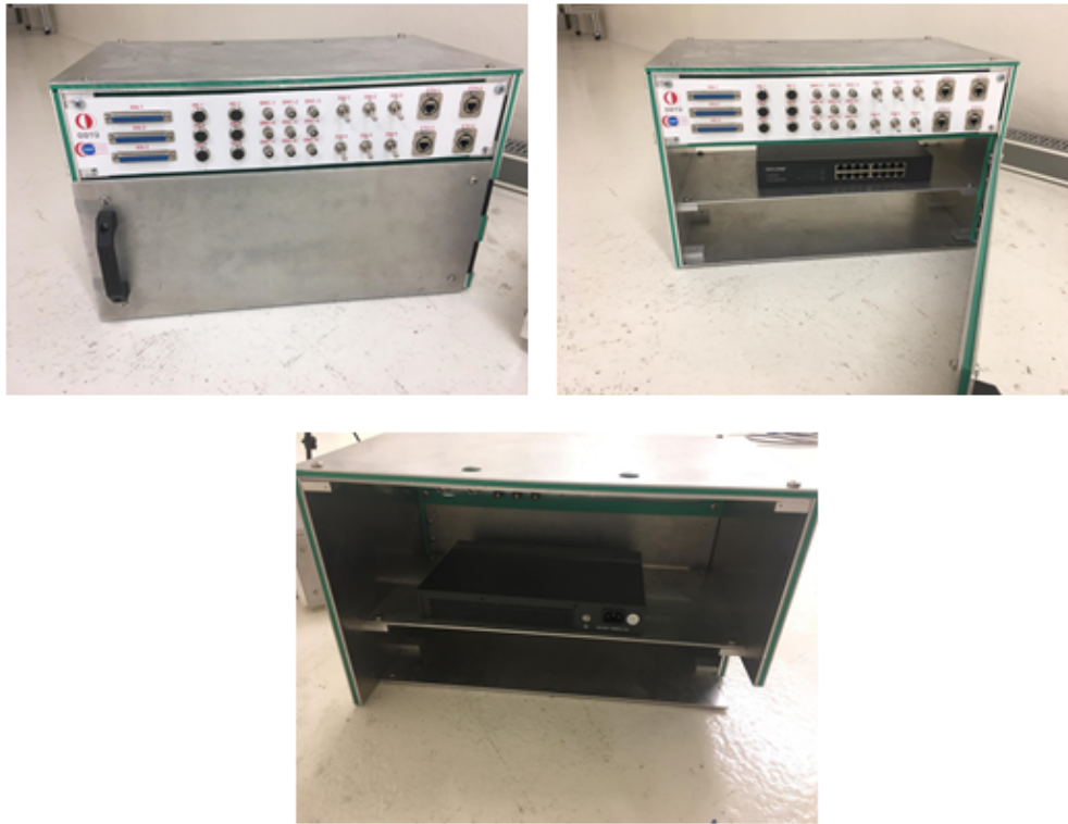
Figure 4.19: Two images from the front (upper panel) and one image from the back (lower panel) of the electronics box of control subsystem are shown. Shielding is Al: 0.50 cm - PE: 1.00 cm from the outside to the inside [108].
