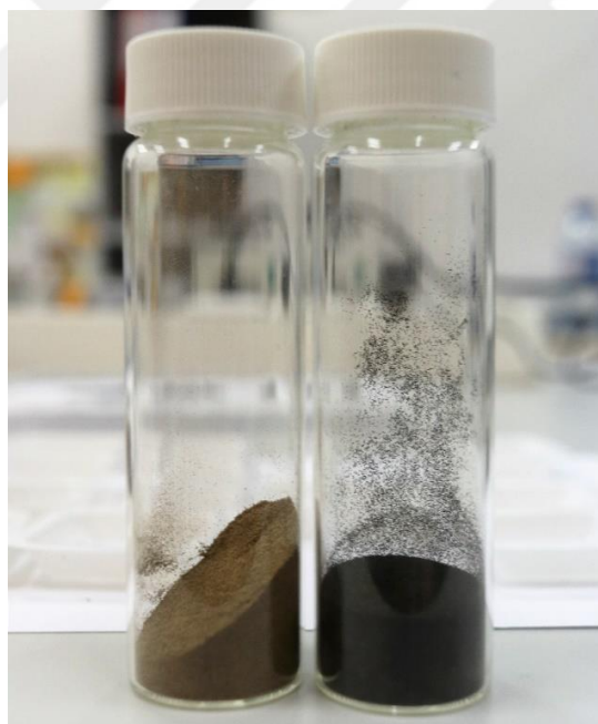
Figure 3.1. Processed Fuel Samples of Olive Residue and Tunçbilek Lignite with size range 106-125 \mu\text{m} for Horizontal Mesh Configuration
