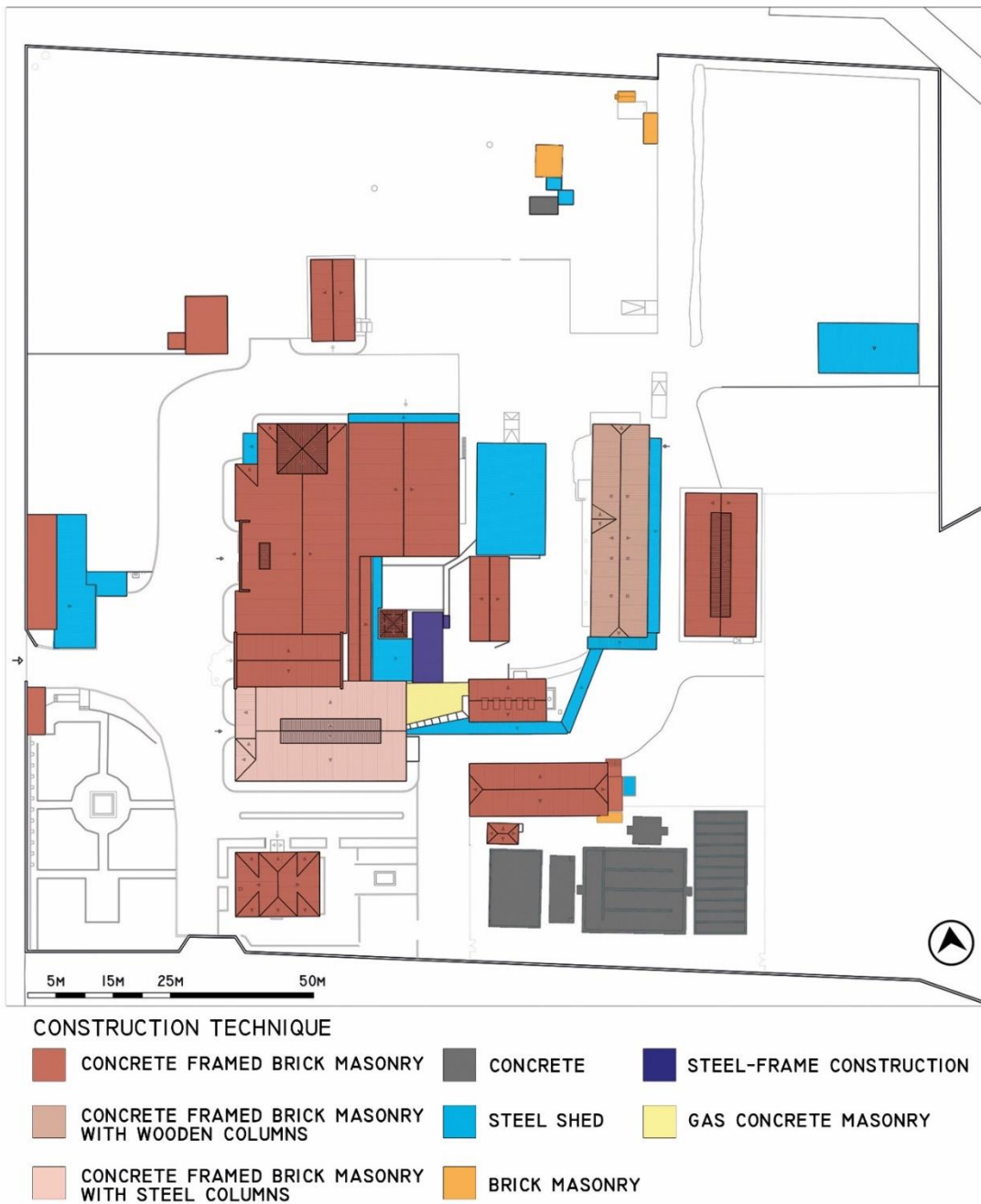
Figure 3.142. The construction technique of the buildings
