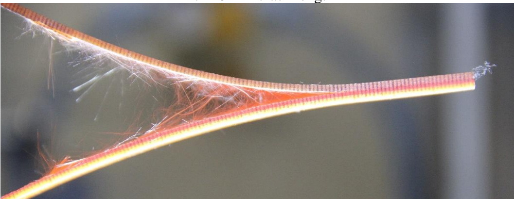
Figure 3.56. Side view of specimen #3 (G-DCB-ENF-65-65-3-MF12060) during DCB test
