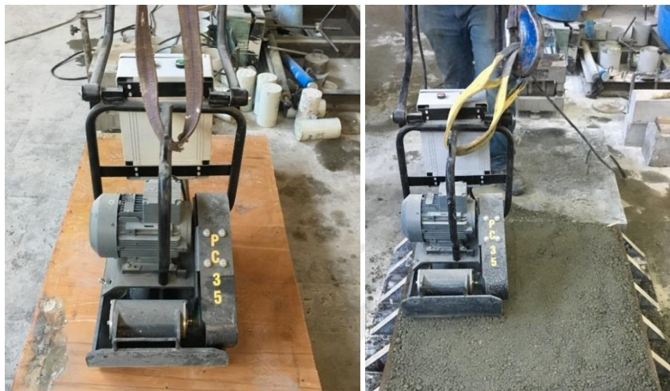
Figure 3.16. Vibratory plate compactor (VPC) application representing field paver compaction process prior to DDVHR application for RCC mixtures
