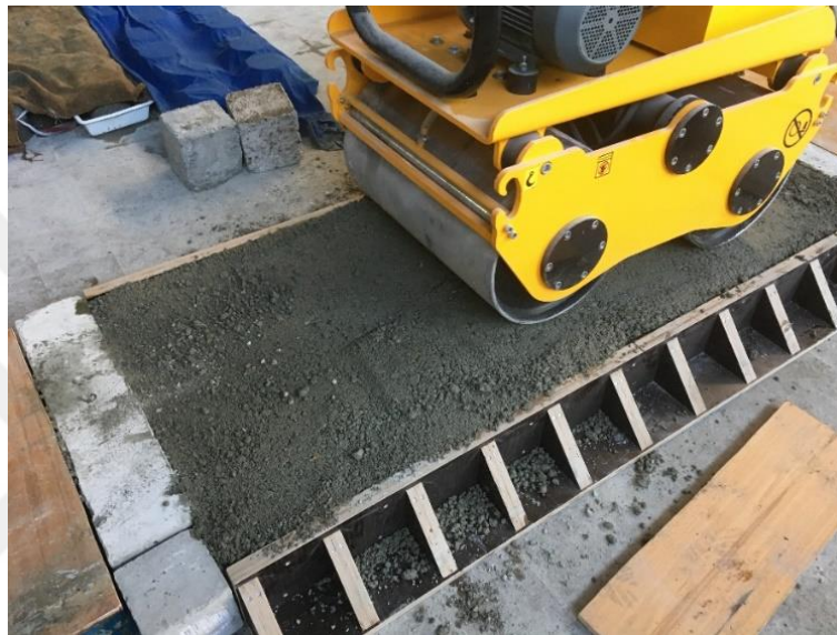
Figure 3.18. Surface undulations for some RCC mixtures during DDVHR application
