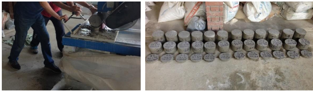
Figure 3.10. Specimens for 28-day compressive strength (ASTM C29), splitting tensile strength (ASTM C496) and density, water absorption and voids in hardened concrete (ASTM C642)
