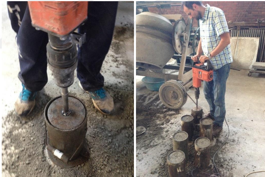
Figure 3.6. Compaction of RCC mixtures by vibrating hammer method (ASTM C1435).
