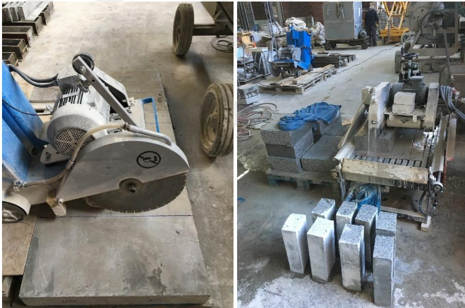
Figure 3.30. RCC plate prepared for fatigue test and test specimens of 10 \times 15 \times 35 \text{ cm}^3 cut from plate (C400-D12-W5.5)
