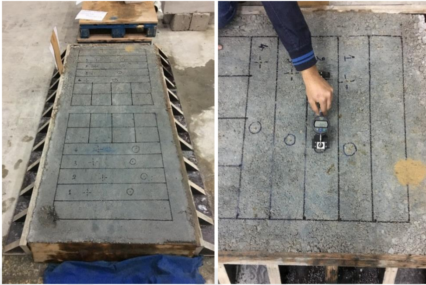
Figure 3.19. Shrinkage measurements on RCC road produced in the laboratory
