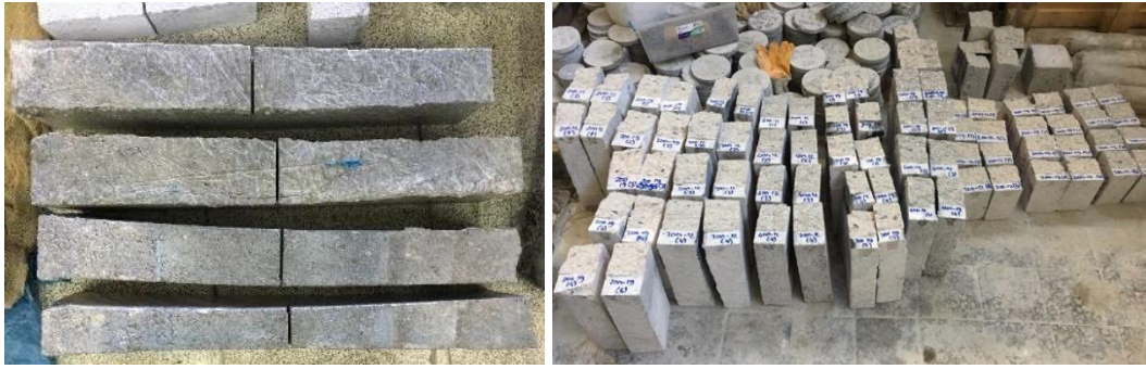
Figure 3.28. Some RILEM beam samples that could not be adequately obtained due to difficulties encountered during cutting and sample views after the test
