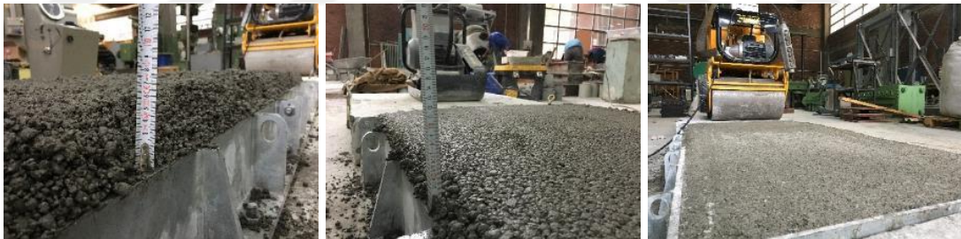
Figure 3.21. Application of VPC and DDVHR for RCC mixtures in the second phase of experimental study
