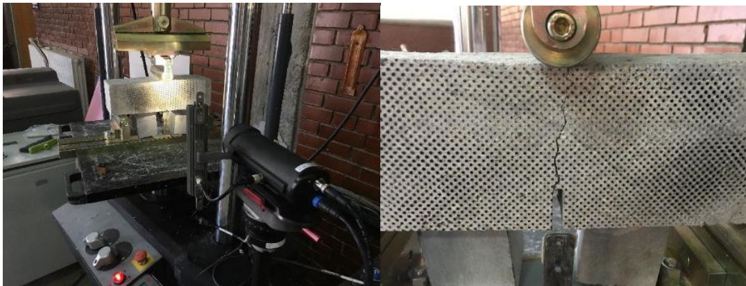
Figure 4.28. Determination of fracture energy of RCC mixtures by three-point bending test applied on notched beam according to JCI-S-001-2003 standard
