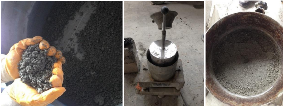
Figure 3.4. RCC mixture consistency and applied Vebe test
