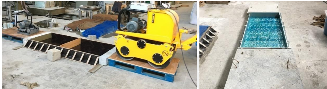
Figure 3.15. Wood and steel molds used for DDVHR
