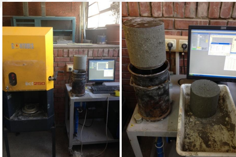
Figure 3.8. Compaction of RCC mixtures by SGC method.
