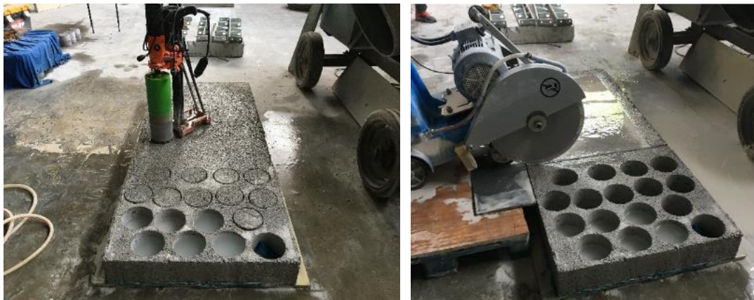
Figure 3.26 Taking the cores on the RCC plate and reducing the plate sizes with walk-behind concrete saw cutting machine
