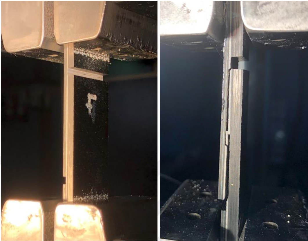
Figure 5.16. Uncracked and cracked specimen
