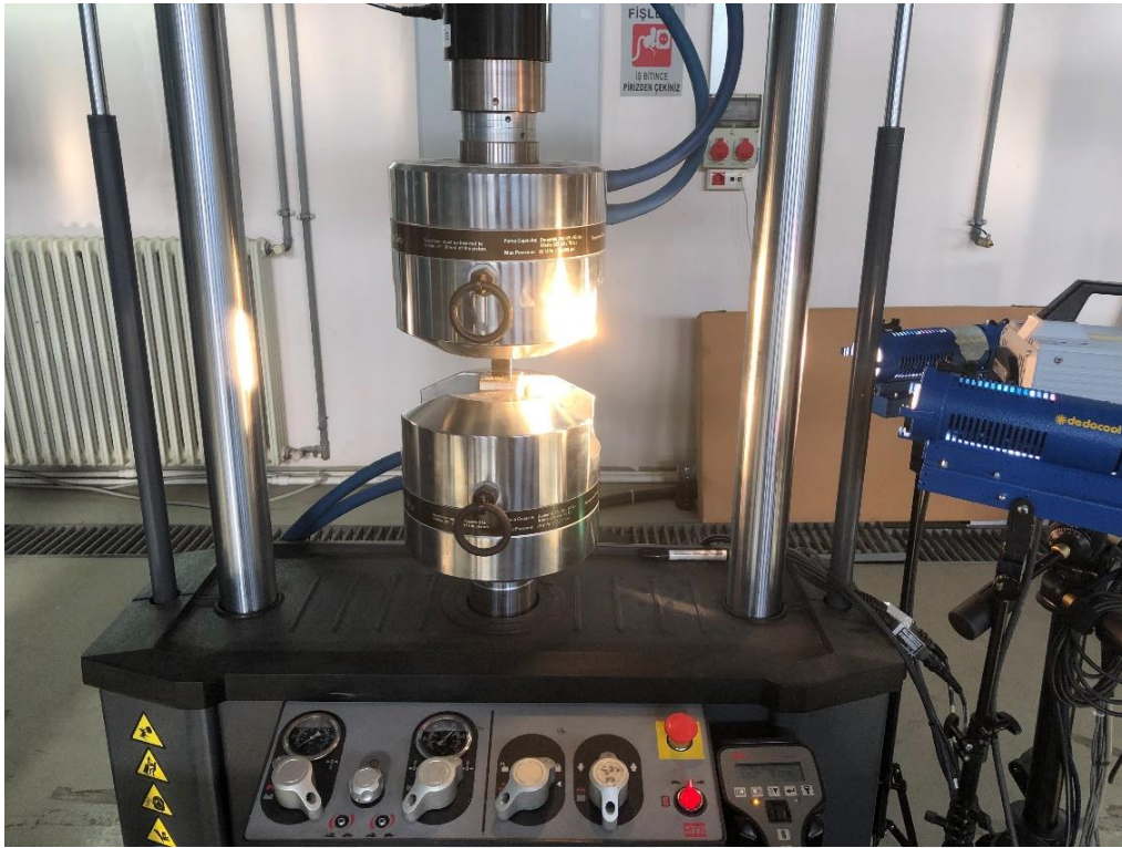
Figure 5.13. SLJ test and high-speed camera setup
