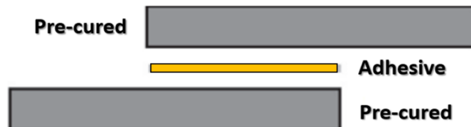
Figure 2.3. Secondary bonding process
