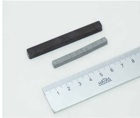
Figure 4.18. Expansion Specimen before and after sintering
