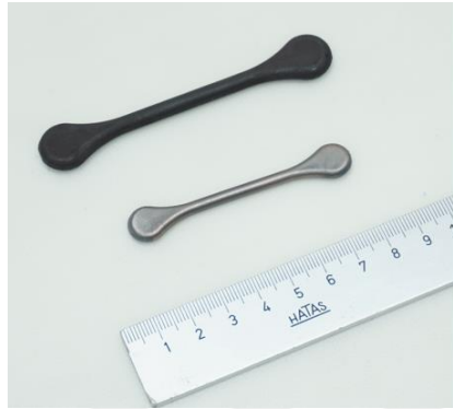
Figure 4.14. Tensile Specimen before and after sintering
