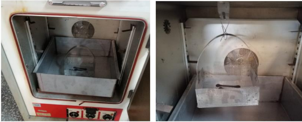
Figure 3.18. Water Debinding Operations
