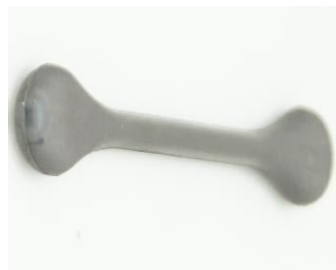
Figure 4.4. Excess material around the molded part
