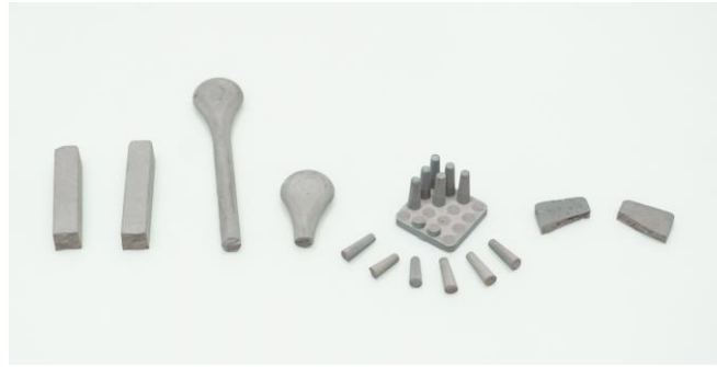
Figure 4.11. The easily broken sintered w-15Cu parts.
