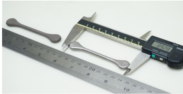
Figure 4.22. Tensile Specimen before and after sintering
