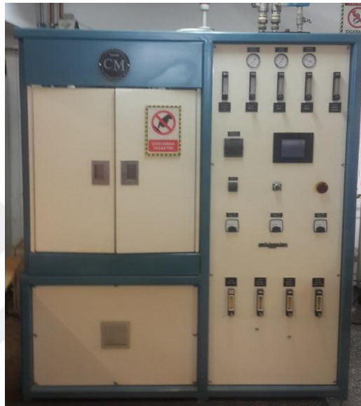
Figure 3.22. Sintering Furnace, CM 1512 H2 GS FL
