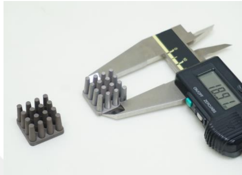
Figure 4.20. Heat Sink Part before and after sintering
