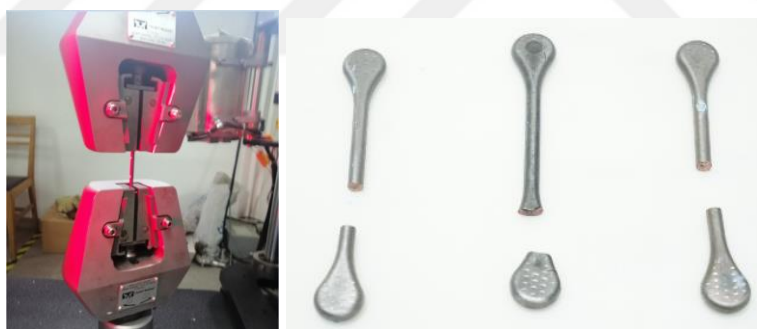
Figure 4.50. Experimental Tensile Test Setup and fractured samples
