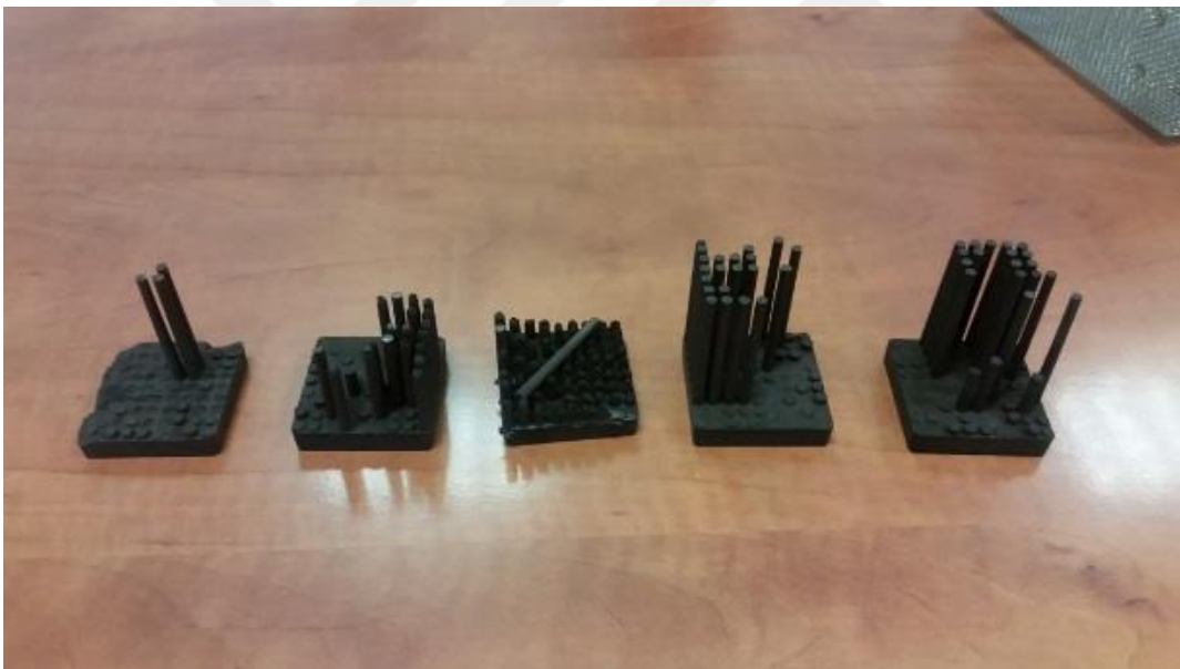
Figure 4.1. Injected heat sink 9x9 with defects.
