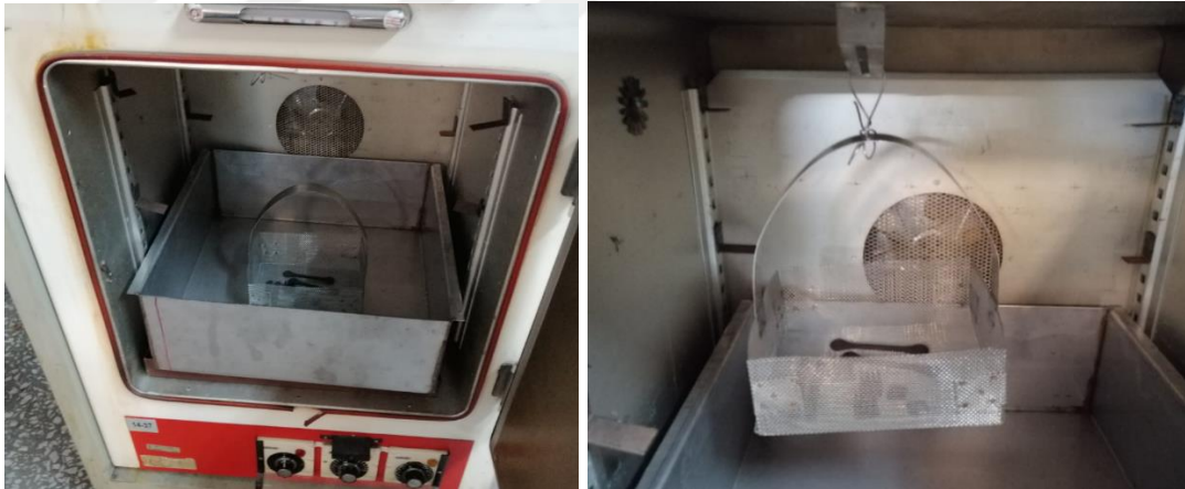
Figure 3.20. Solvent Debinding Operations
