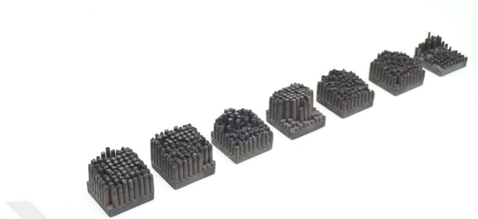
Figure 4.3. Injected short finned version of heat sink 9x9 with defects.
