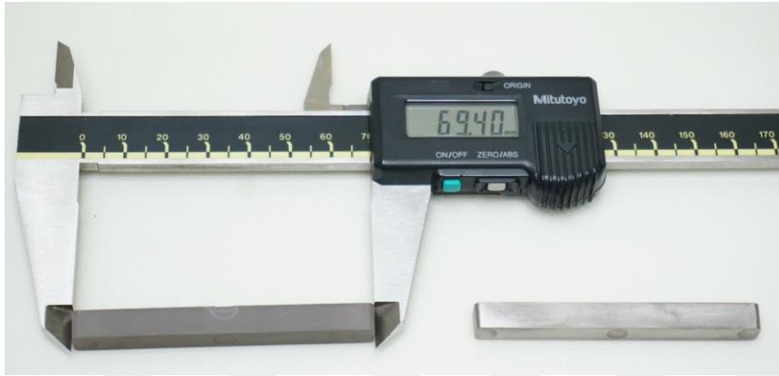
Figure 4.26. Expansion Specimen before and after sintering
