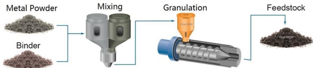
Figure 2.33. Feedstock Preparation Steps
