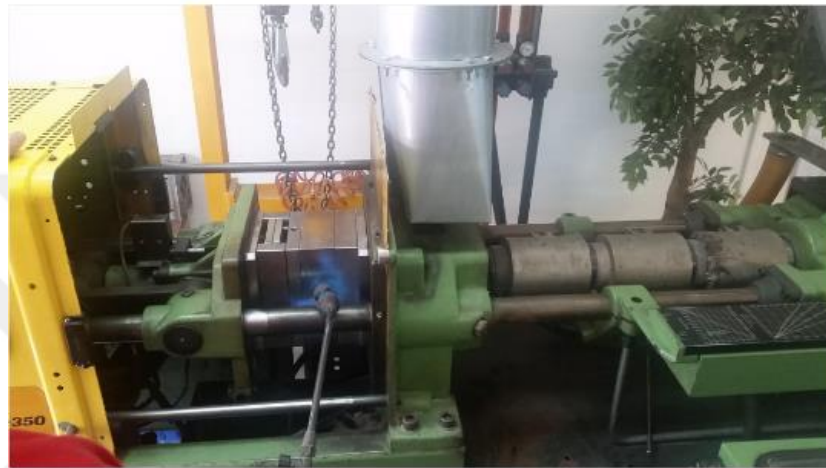
Figure 3.15. Mold assembled to the Injection Molding Machine
