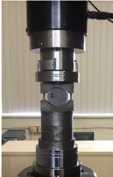
Figure 5.7. The indirect tensile strength test configuration for 54 mm diameter with jaws
