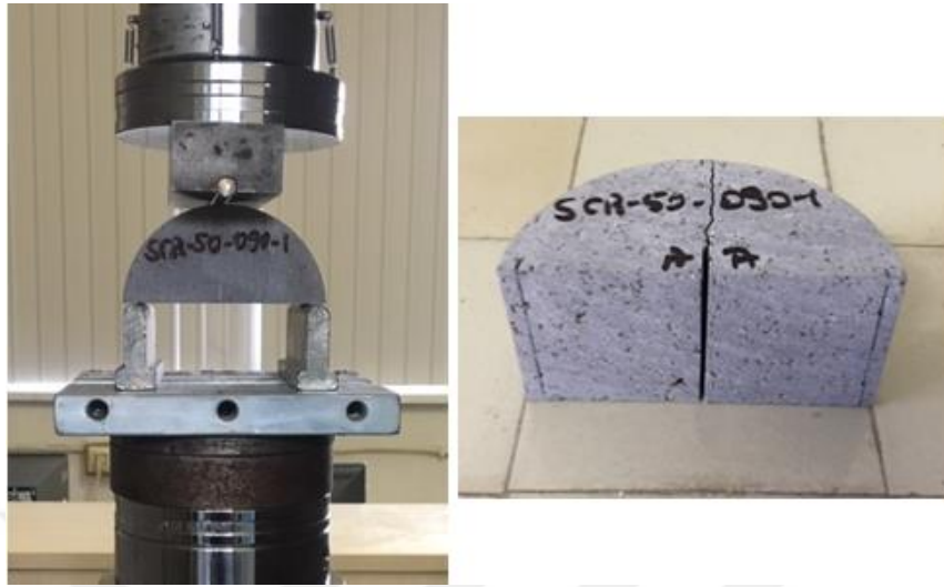
Figure D. 79. SCB-50-090-1 specimen during and after test
