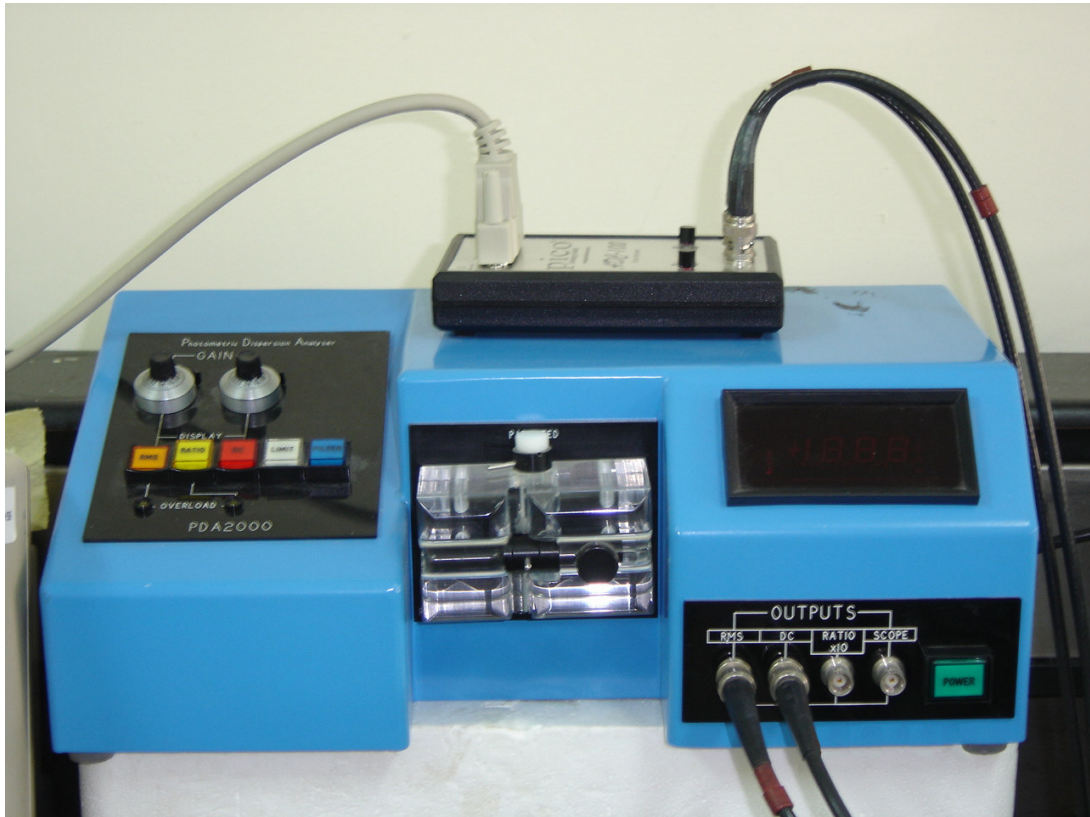
Figure-III.2: Photometric Dispersion Analyser (PDA 2000, Rank Brothers Ltd., Cambridge, UK).
