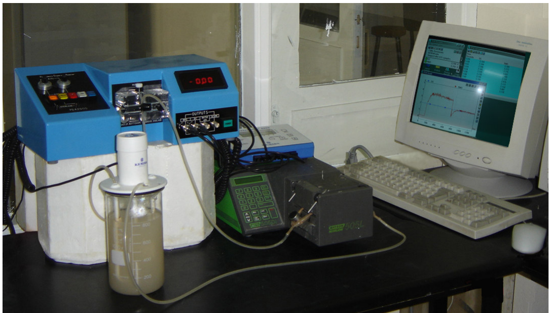
Figure-III.6: Experimental setup for dynamic monitoring of floc formation in jar-test procedure.
