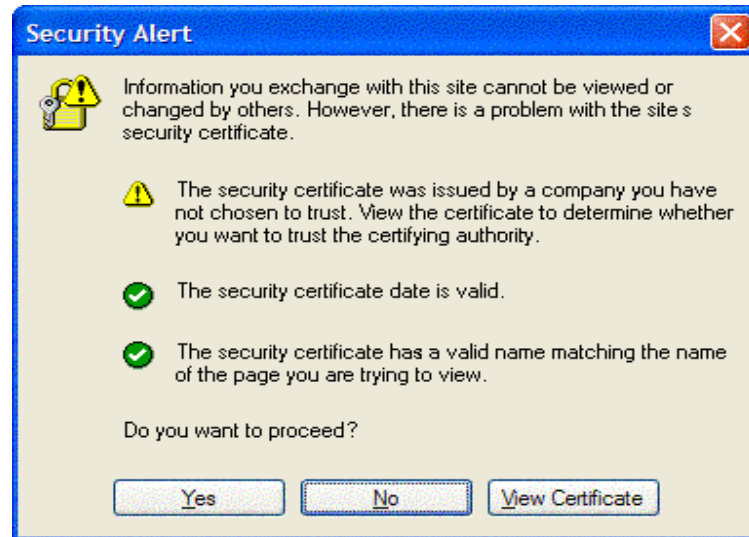
Figure 2 : Warning message when the certificate is not in the browser's trust list
