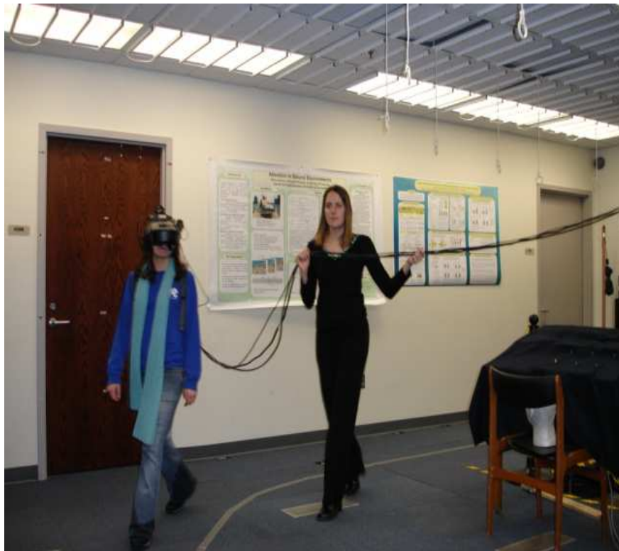
Figure 4-6 Virtual Research V8 Head Mounted Display with 3rd Tech HiBall Wide Area motion tracker
