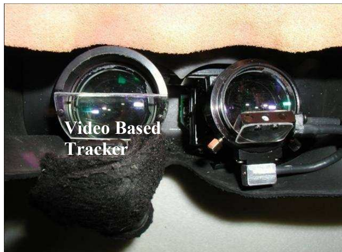
Figure 4-4 - V8 optics with ASL501 Video Based Eye Tracker (Left)
