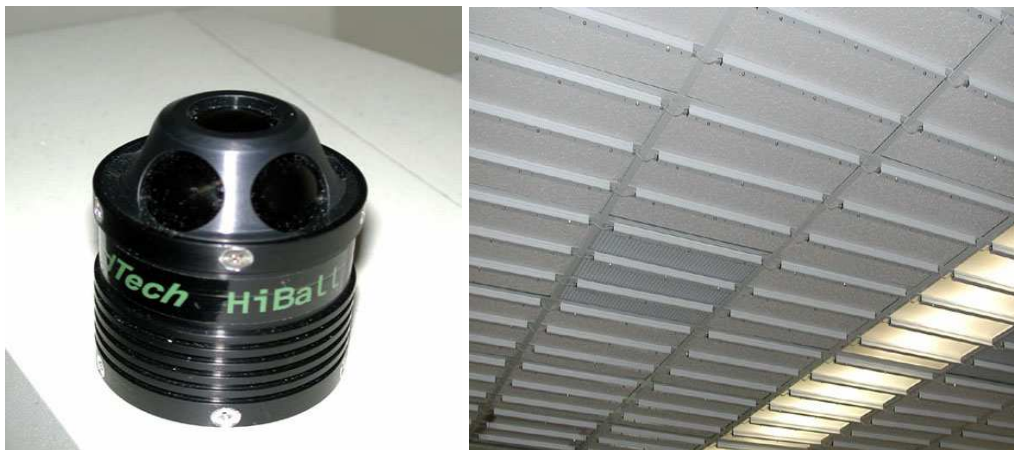
Figure 4-5 First picture shows the Hi-Ball sensor and the second picture shows the Hi-Ball ceiling mounted positional array. Each unit contains 8 Infrared Emitting Diodes that are activated over a high speed network.
