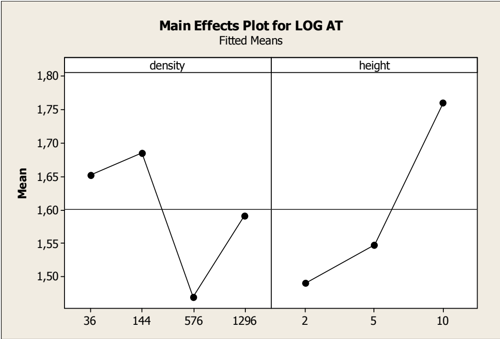
Figure 24 Hover: Main Effects Plot for LOG AT versus Object Height (3 levels), Object Density (4 levels)
