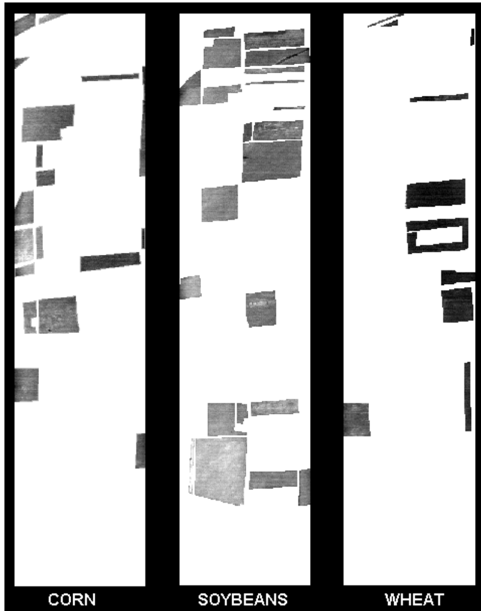
Figure 5.4 – Ground Truth Masks of corn, soybeans and wheat classes extracted from spectral band 1 image.
