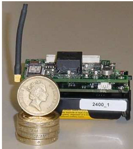
Figure 1.2: A real sensor node example, MicaZ [20] with dimensions 58mm \times 32mm \times 7mm excluding the battery pack
