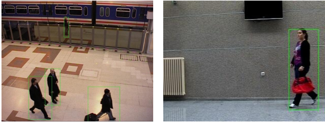
Figure 3.9: An example result of adaptive mean shift for automated multi object tracking in visible domain
