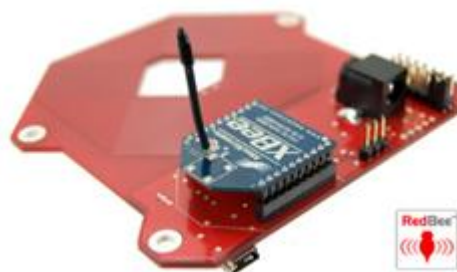
Figure 4.7 - Redbee RFID Reader
