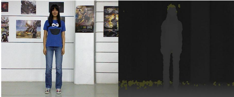
Figure 2.3: Depth Data Stream of Kinect Left: RGB Image Captured with Kinect's Color Camera Right: Depth Image Stream Captured with Kinect's Depth Camera
