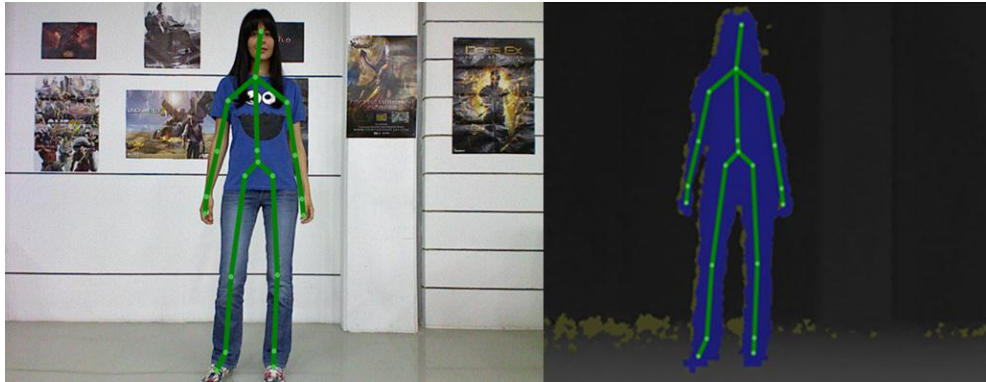
Figure 2.4: User Skeleton Recognized by Kinect Left: RGB Image Showing Tracked Skeleton Right: Depth Image Showing Tracked Skeleton
