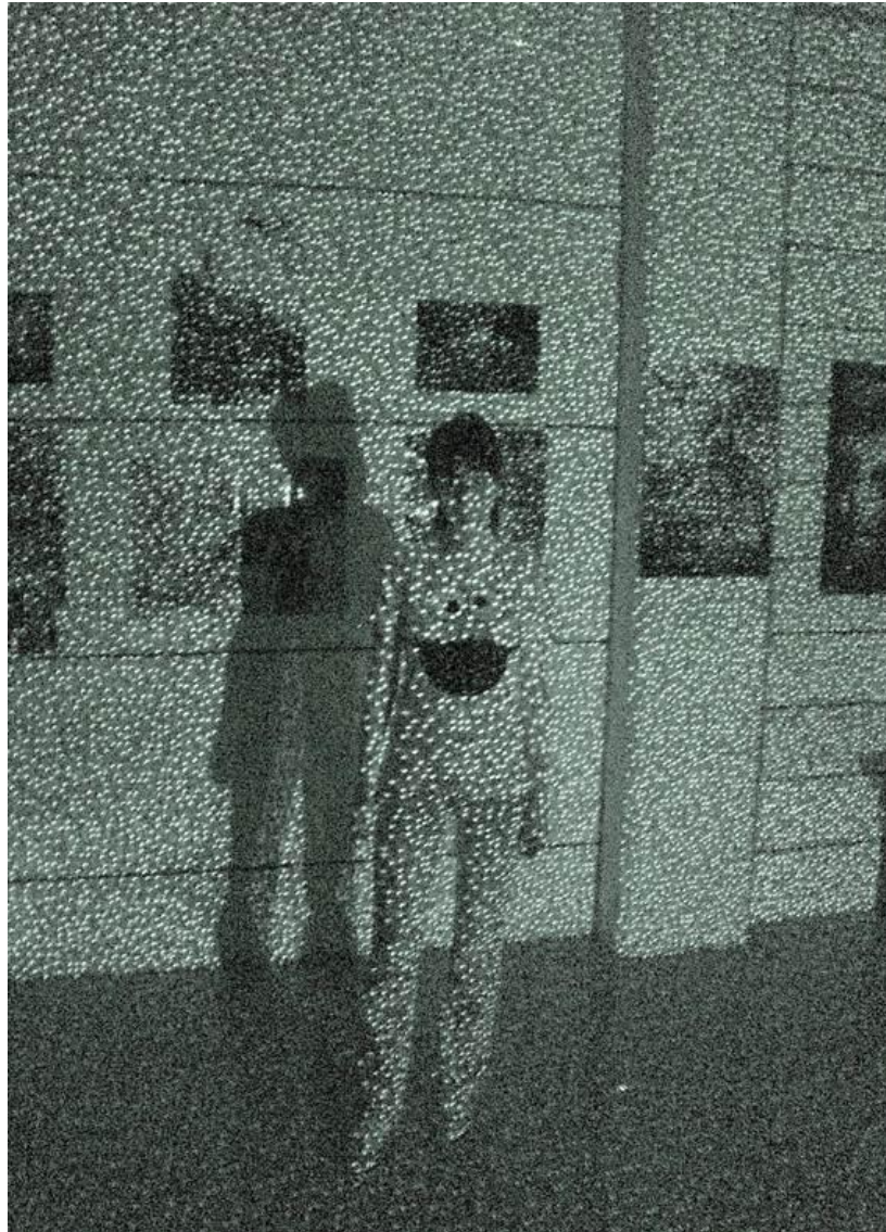
Figure 2.2: IR Rays Cast Out by Kinect to Detect Depth Information
