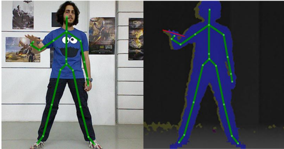
Figure 3.5: Detection of the Hand Rotation from Depth Data Left: RGB Image of the Player Directing His Right Hand towards Kinect Right: Depth Image of the Player with Right Hand Rotational Direction Detected
