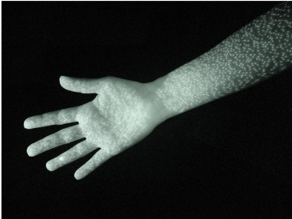
Figure 2.9: Infrared Rays Scattered from Depth Camera Impinging on the Arm
