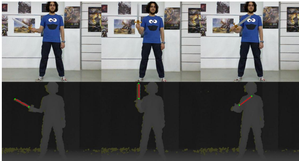
Figure 3.11: Player Rotates the Sword in Rolling Axis of Motion Left: Player Leans the Sword Right in Global z Axis Middle: Player Holds the Sword Perpendicularly Right: Player Leans the Sword Left in Global z Axis
