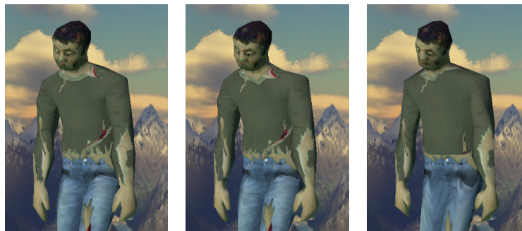
Figure 2.3: Discrete geometric detail level meshes of the same character with 652, 548 and 382 polygons
