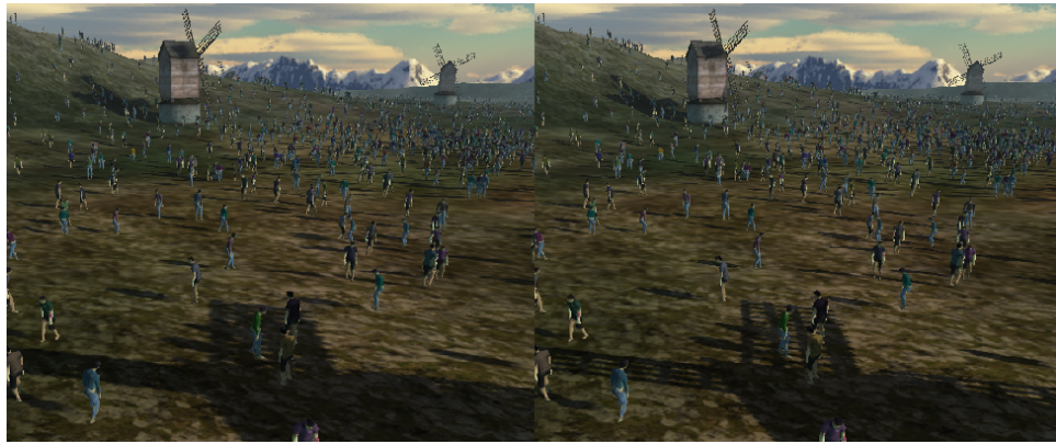
Figure 4.5: Left: 1 cascade 2048x2048 Shadowmap, Right: 4 cascades of 1024x1024 shadowmaps. Better shadowing quality achieved while same amount of texture memory being used.
