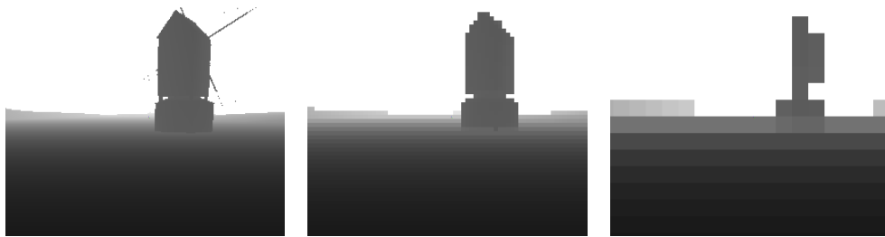
Figure 4.2: Illustration of the 3 mip levels of hierarchical-z buffer
