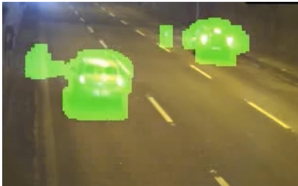
Figure 6: A state of the art background subtracting output that fails in tunnel environment
