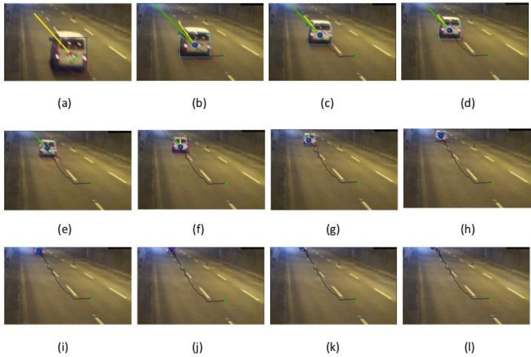
Figure 11: Successful tracking of a car during the consecutive frames a-l using the optical flow method
