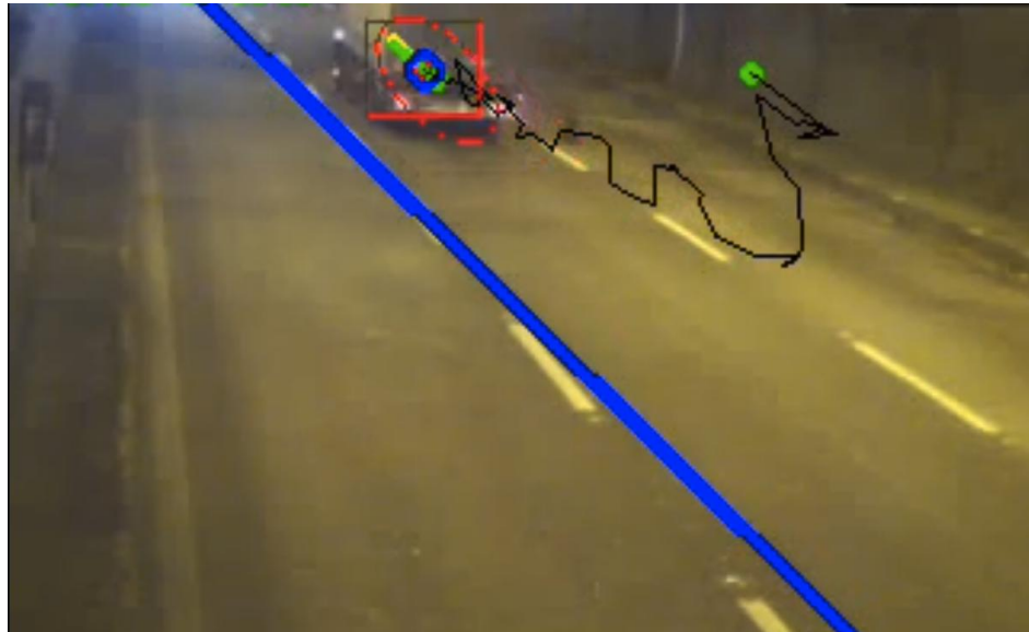
Figure 7: A state of the art tracking output that fails in the tunnel environment
