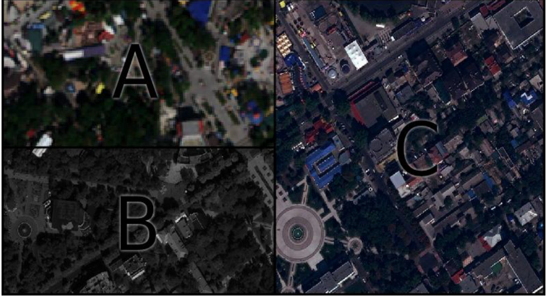
Figure 4.2: The result of pansharpening algorithm (A: Multispectral Image, B: Panchromatic Image, C: Pan-sharpened image)
