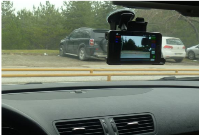
Figure 49 Convenient mounting for a correct camera view
