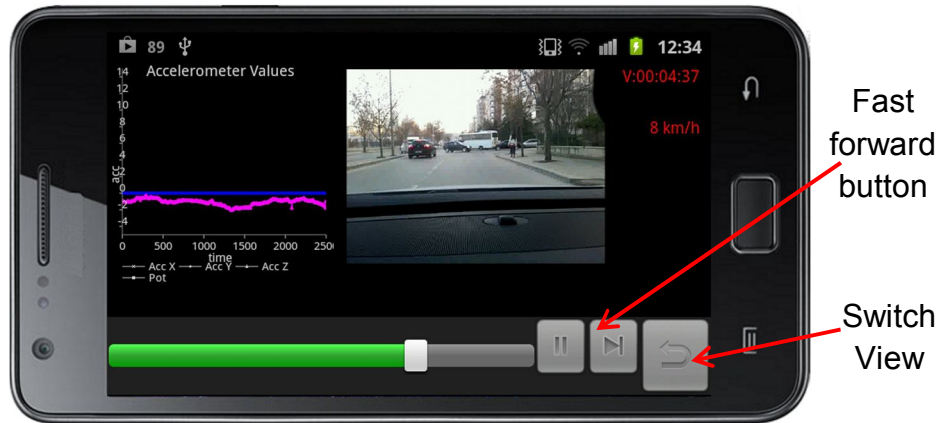
Figure 42 Replay mode: video and sensor values positions are synch
