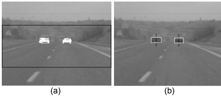
Figure 11 Object Detection on the extracted region of interest: (a) darker regions are identified and (b) the objects are filtered according to their dimensions
