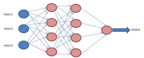
Figure 8: Structure of an artificial neural network. (Adapted from Data Mining: Concepts and Techniques. Jiawei Han, M. Kamber. 2001)
