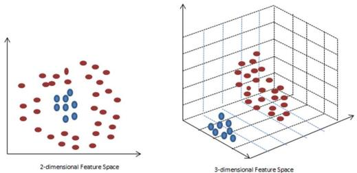
Figure 10: Matching two dimensional space onto three dimensional by Kernel Trick. (Adapted from Support Vector Machines Explained by Tristan Fletcher. UCL 2009)
