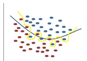
Figure 2: Overfitting Problem: The model memorizes the training dataset and so unable to make a generalization on different dataset of the same problem. (Adapted From: Model Selection and Multimodel Inference. A Practical Information-Theoretic Approach. Burnham
