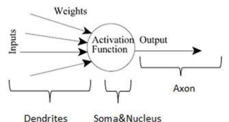
Structure of an artificial neuron (Adapted from Data Mining: Conce
