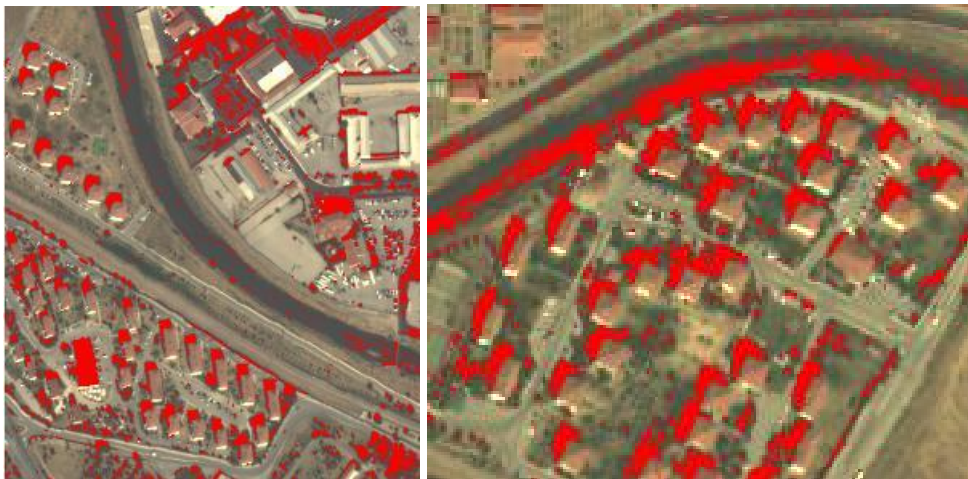
Figure A.27: Ratio based on YC_bC_r color space on true color image
