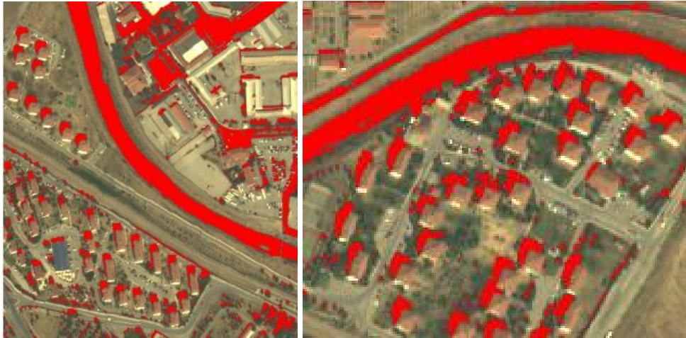
Figure A.26: Ratio based on YUV color space on false color image
