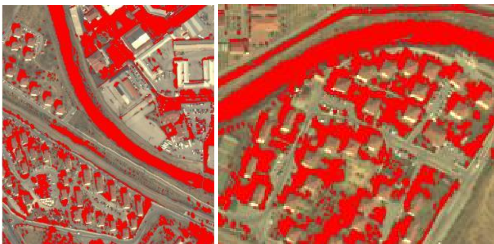
Figure A.17: Ratio based on saturation and intensity on true color image
