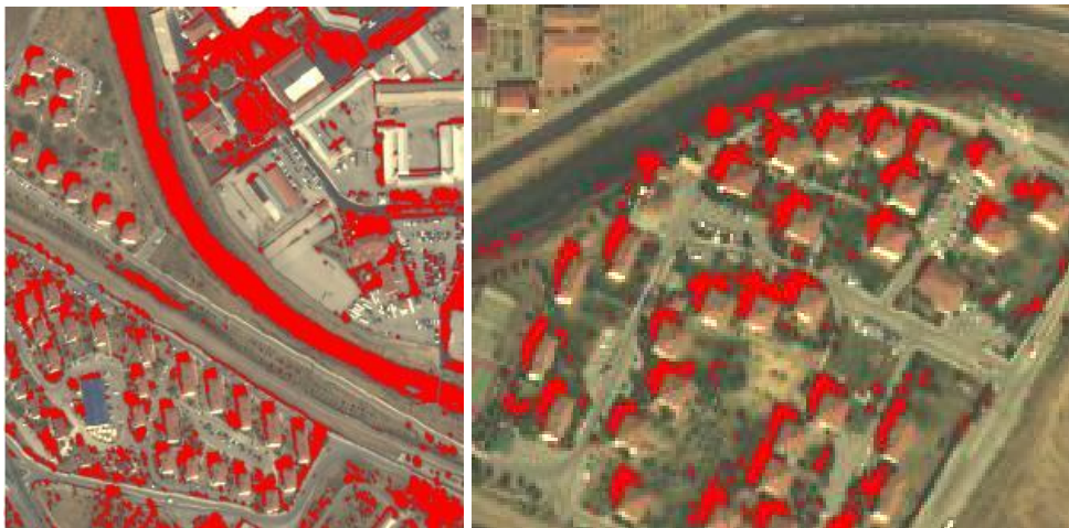
Figure A.21: Ratio based on HCV color space on true color image
