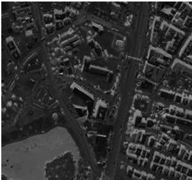
Figure 4.8: Tsai's ratio map of the false color image on HSI color space
