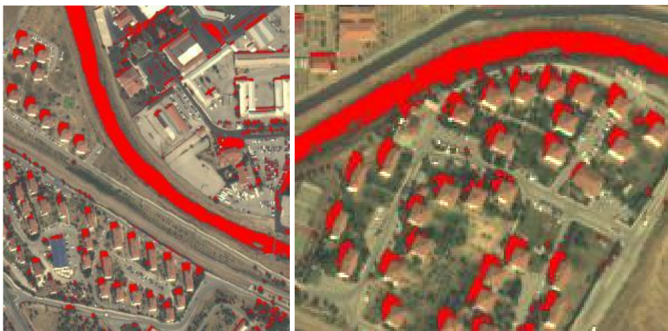
Figure A.22: Ratio based on HCV color space on false color image
