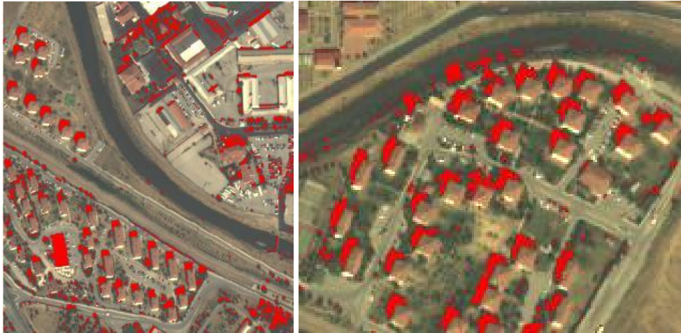
Figure A.23: Ratio based on C_1C_2C_3 color space on true color image
