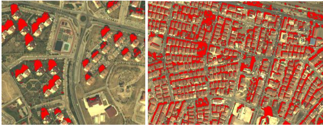
Figure A.6: Ratio based on HCV color space on true color image
