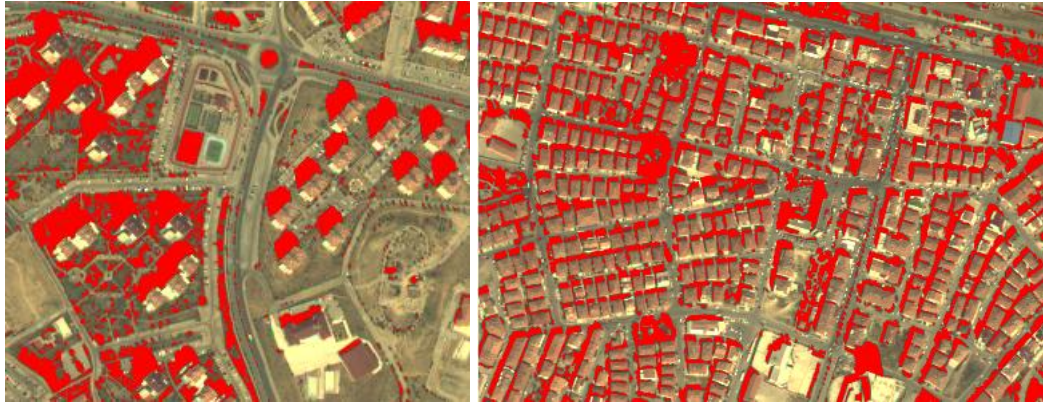
Figure A.2: Ratio based on saturation and intensity on true color image
