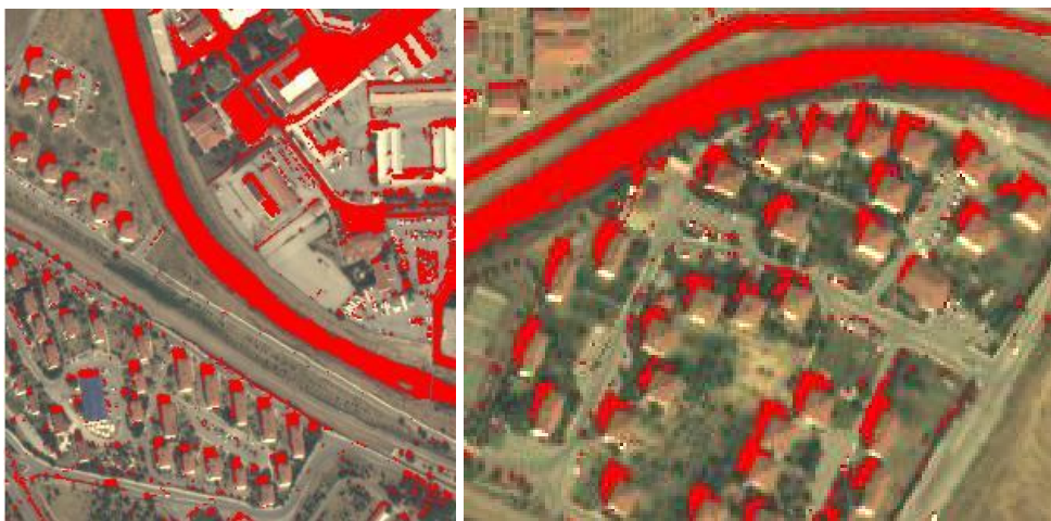
Figure A.28: Ratio based on YC_bC_r color space on false color image
