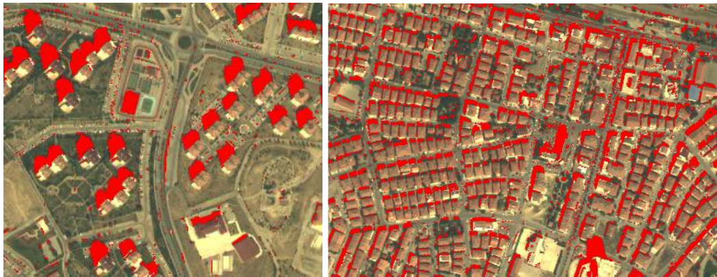
Figure A.13: Ratio based on YCbCr color space on false color image
