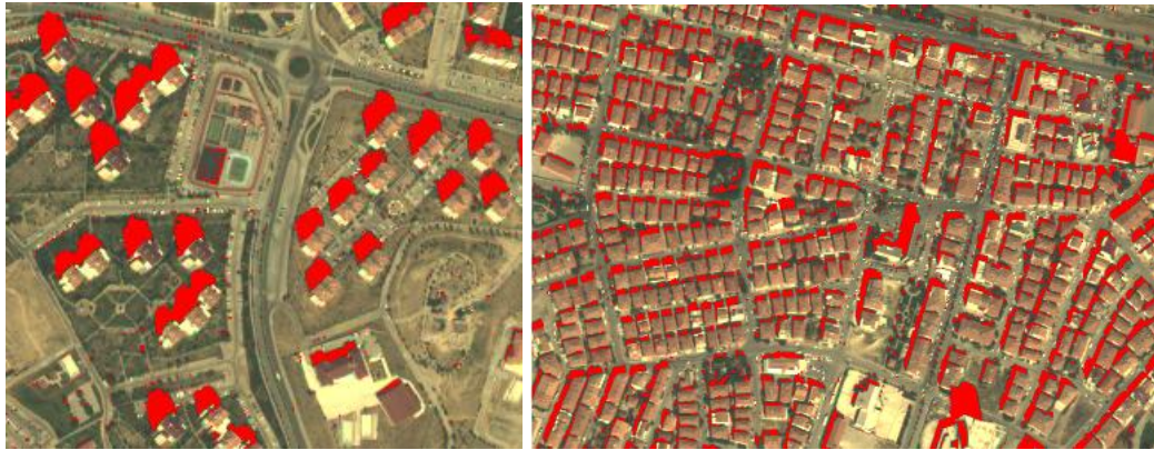
Figure A.9: Ratio based on C_1C_2C_3 color space on false color image
