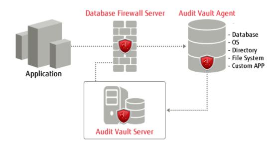
Figure 3.4: Oracle Audit Vault Working Principle
