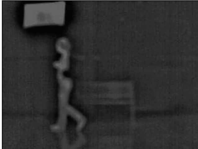
Figure 1 A thermal image acquired with a Long Wave Infrared Camera covering the spectral range 8-12 micrometer [1]
