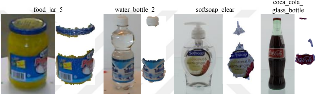
(b) Sensor fail to capture transparent surfaces.
