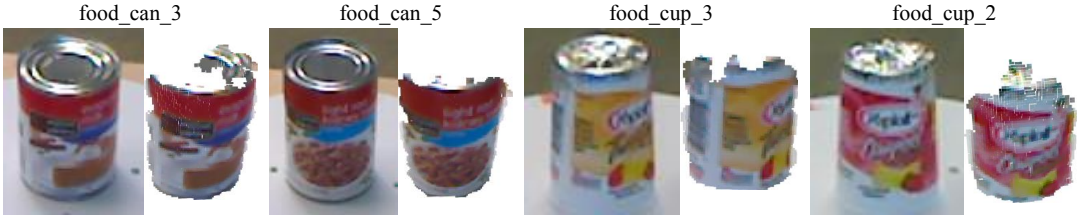
(a) Sensor fail to capture metallic surfaces.
