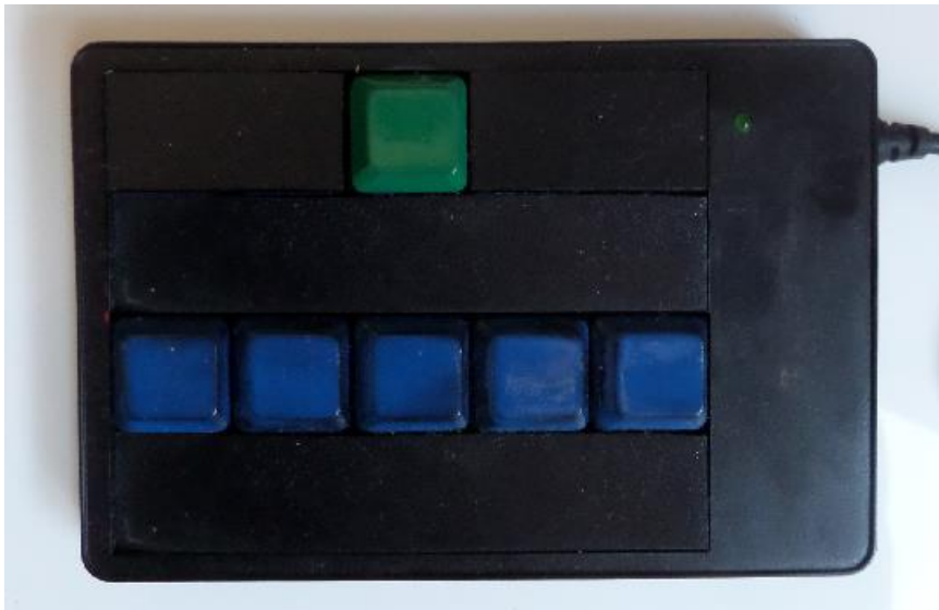
Figure 16: Numpad that is designed and used in m-BART. The fundamental aspect of the keyboard is that it helps participant to control the keyboard without looking to it. The single button on the upper row pumps all balloons, and the buttons on the lower row collects rewards respectively.
