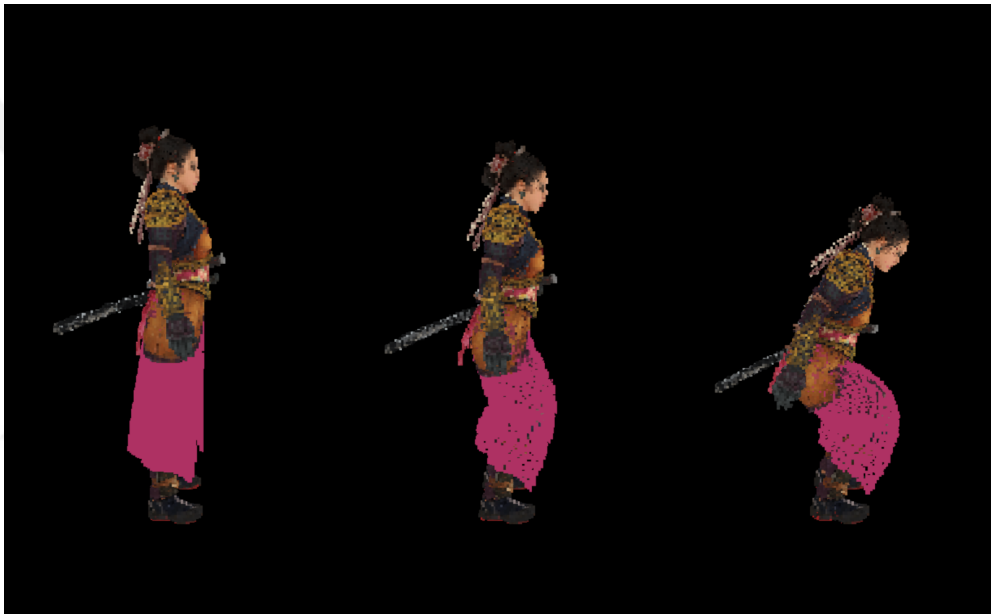
Figure 4.14: Nyra character doing her jumping animation. First frame is the characters bind pose and there is no inconsistency of voxels. However after key-frame interpolation, transformation artefacts occur because of the method limitation.
