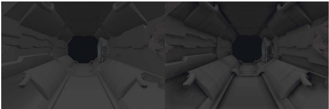
Figure 2.5: SSAO example from Cry Engine 2. Notice the darkened pixels near hard edges [41].
