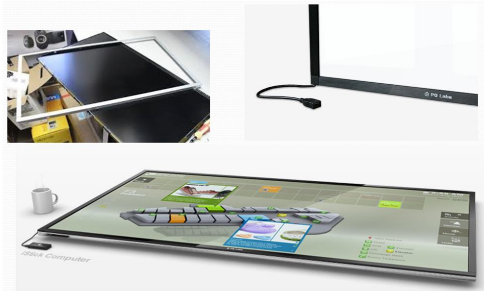
Figure 2: Construction of the Large-Size Screens
