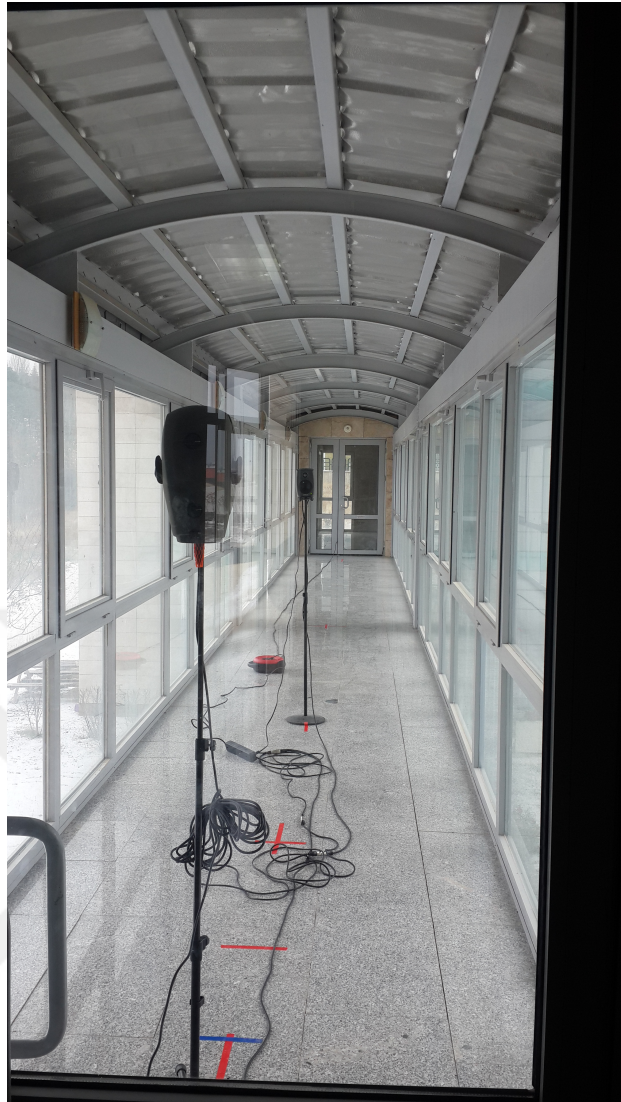
Figure A.2: The hallway used for recording binaural room impulse responses
