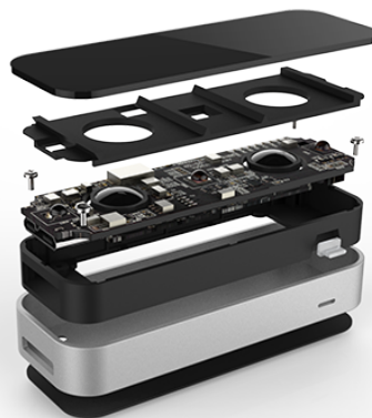
Figure 2.4: Leap Motion Decomposition. Image Courtesy of Leap Motion [4]
