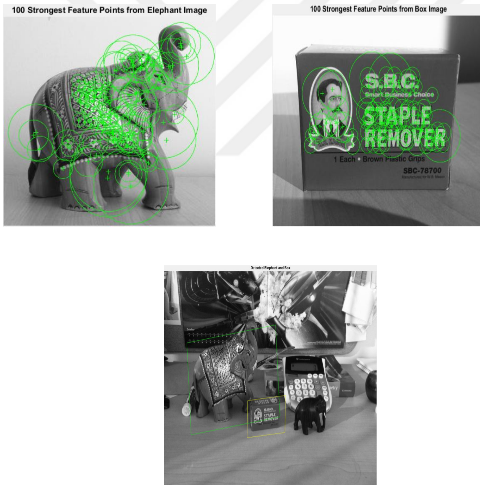
Figure 2.3: Object Detection example. Elephant and box features are extracted. They are detected in the whole scene. This figure is a reproduction using Matlab toolbox object detection example code.
