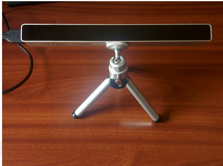
Figure 3.2: EyeTribe eye tracker device used in thesis
