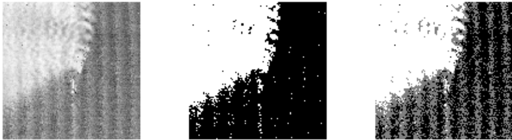
Figure 82 Data cube 1 Detection Results with Algorithm 2 Sulfur Hexafluoride (Otsu)
