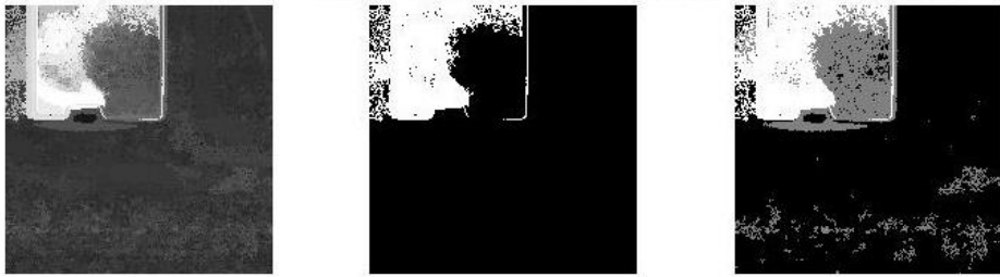
Figure 43 Data cube 1 Detection Results with Threshold 500 (Otsu)
