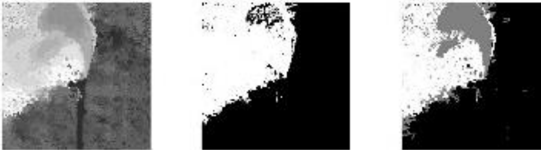
Figure 67 Data cube 2 Detection Results with Threshold 1000 (Otsu) (Sulfur)
