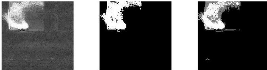
Figure 39 Data cube 1 Detection Results with Threshold 50 (Otsu)
