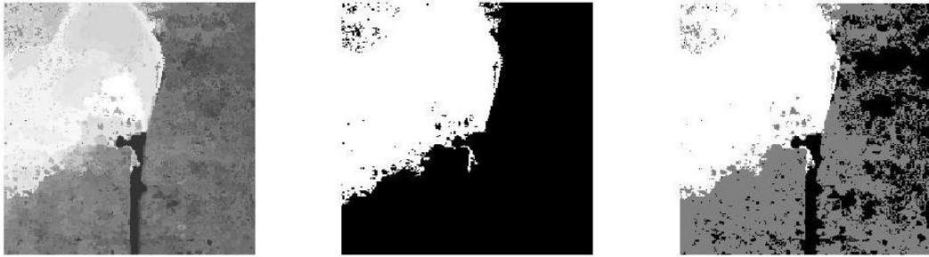
Figure 79 Data cube 2 Detection Results with Threshold 1000 (Otsu) (Ethylene)
