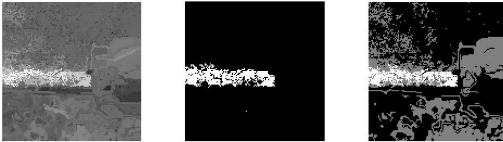
Figure 102 Data cube 3 Detection Results with Threshold 250 (Otsu)
