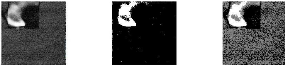
Figure 48 Data cube 1 Detection Results with Algorithm 2 (Otsu)
