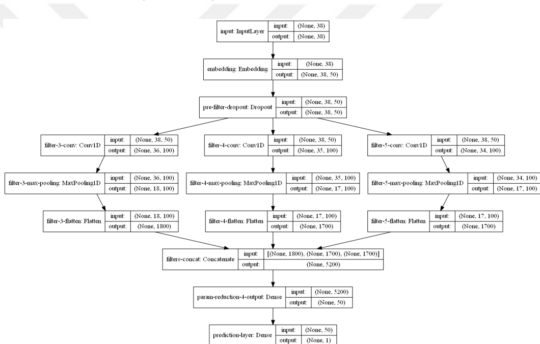
Figure 3.1: Figure showing a potential utilization Convolutional Neural Networks for text classification job (Kim, 2014)
