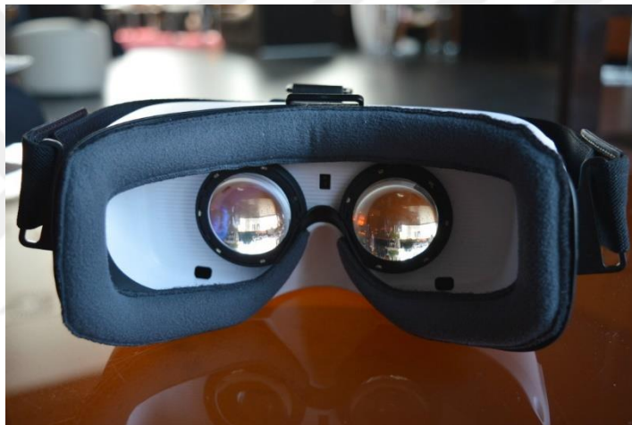
(b) Device back: Infrared lights (around each lens), proximity sensor (in the middle), and the lenses.
