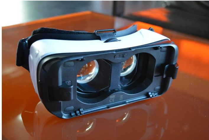
(a) Device front: Eye tracking components (reflectors, cameras) and phone mount.
