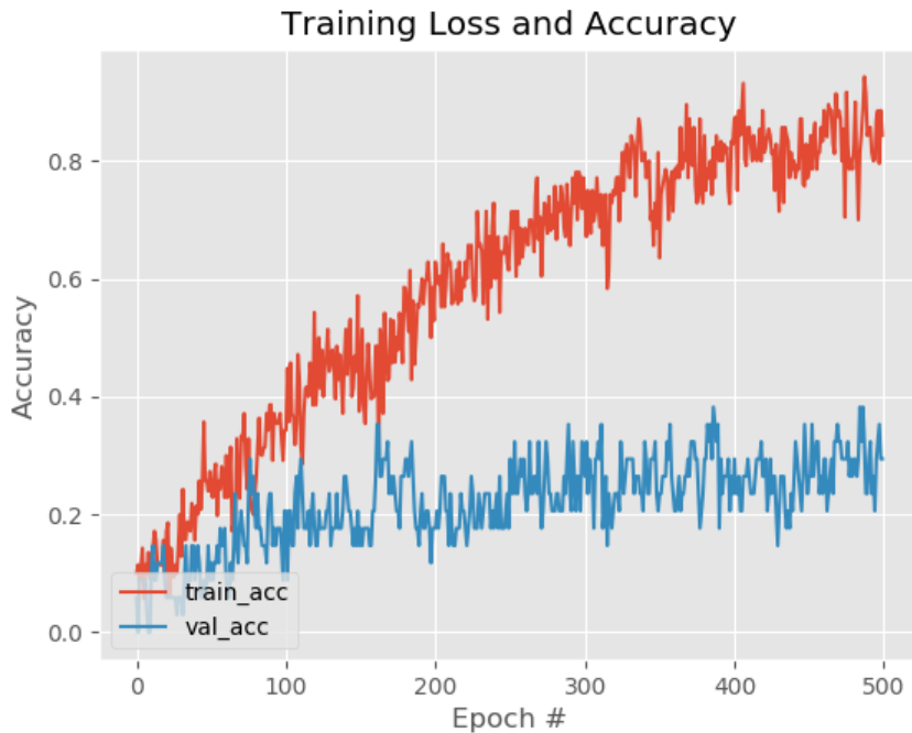
Figure 30: Training accuracy percentages of the constructed ANN model where validation dataset size was increased. Red line represents training accuracy and blue line represents validation accuracy.
