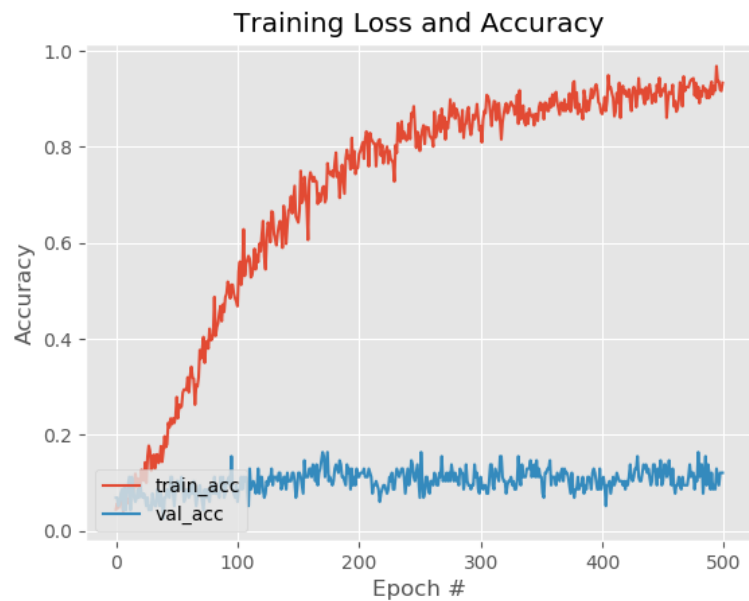
Figure 29: Training accuracy percentages of the constructed ANN model. Red line represents training accuracy and blue line represents validation accuracy.
