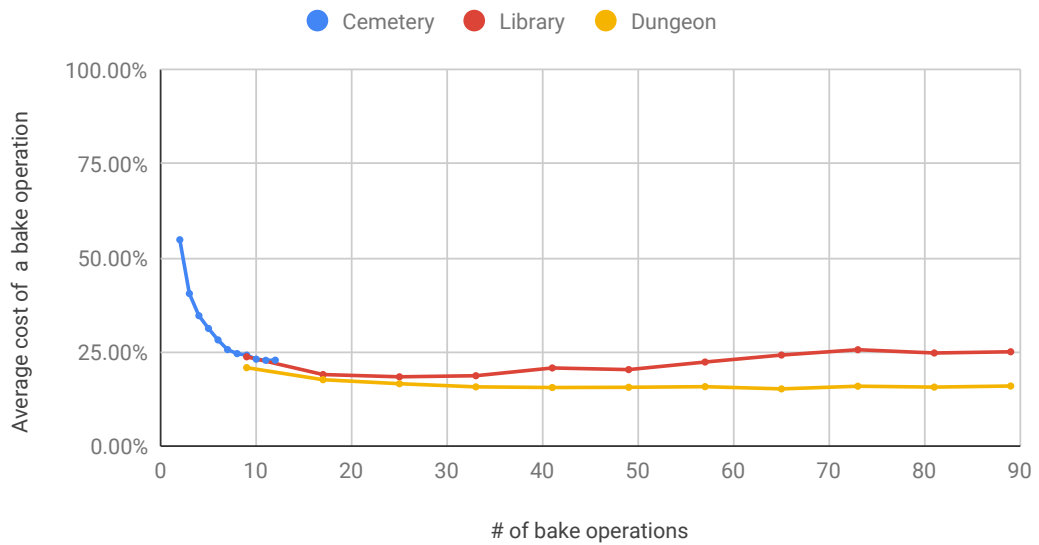
Figure 5.8: Average time spent on a single baking operation significantly decreases as the number of consecutive bake operations increases.
