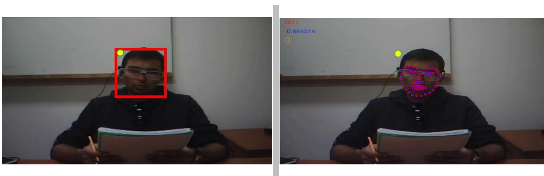
Figure 7: Face detected either in a rectangular shape or with landmark points a)The previous method identified face boundary as a rectangle b)OpenFace detected 68 facial landmarks for positioning the face.
