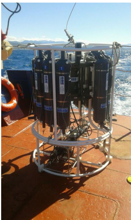
Figure 2.2. 12-bottle Rosette System coupled on CTD probe.
