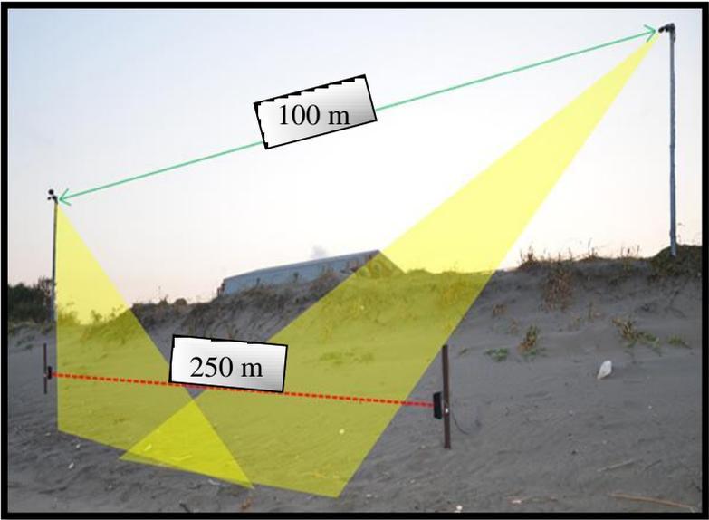
Figure 2.2-13 the illustration showing field of view covered by the camera couple with laser beam
