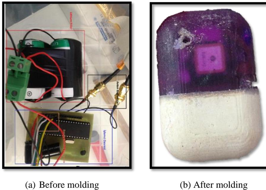
Figure 2.6-2 Tracking system setup before (a) and after (b) molding process
