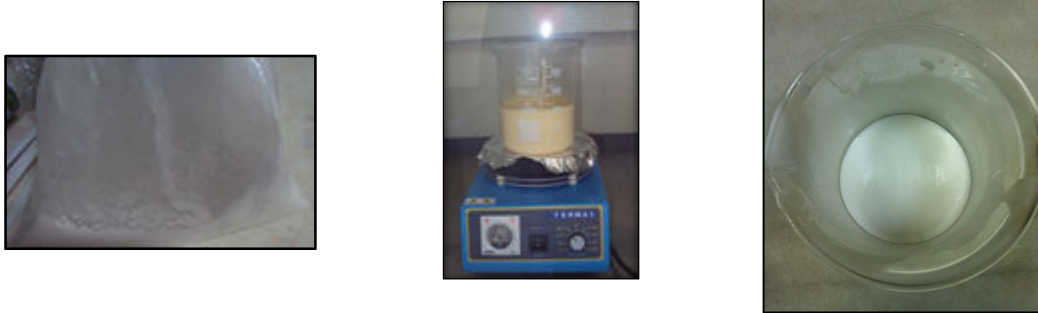
Figure 3.2. Procedure of beneficiation of Seydişehir alumina; a) alumina powder as taken (at left), b) leaching procedure on heating magnetic stirrer, c) After boiling with distilled water and decantation of the excess water.
