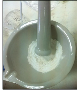
Figure 3.9. Crushing and grinding of bioceramic pellets for XRD powder analysis measurements.
