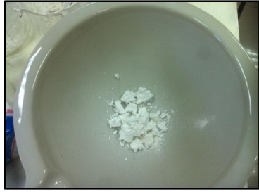
Figure 3.9. Crushing and grinding of bioceramic pellets for XRD powder analysis measurements.
