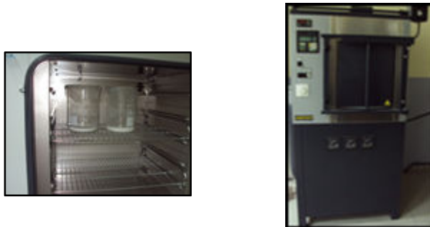
Figure 3.3. Powders of alumina after beneficiation when drying at the drying oven (at left) and when sintering in the furnace (at right).
