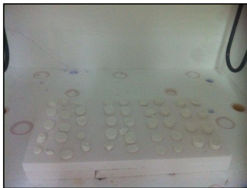
Figure 3.8. Sintered specimens of the first group of -S- type specimens, from left to right, S1 group to S4 group.
