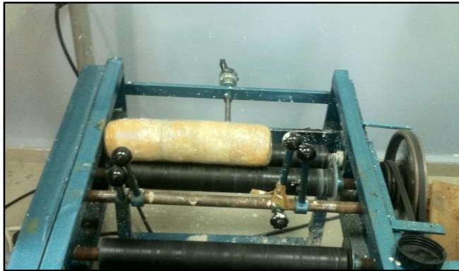
Figure 3.6. The basic ball milling process we applied for grinding and also homogenization of the specimens.
