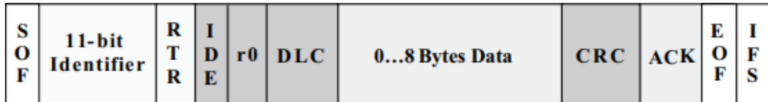
Figure 2.2: Standard CAN: 11-Bit Identifier [4]
