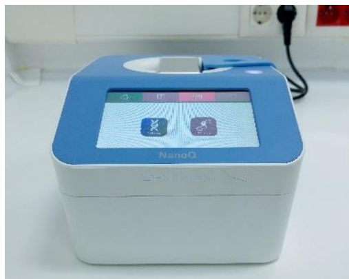
Figure 2.17 Optizen NANO Q Spectrophotometer. dsDNA and protein measurement modes were shown in the figure.
