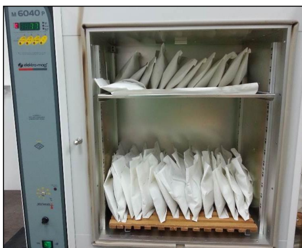
Figure 2.12 Plant parts samples (washed and unwashed leaves, branch, and bark) in oven.
